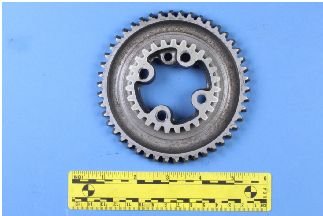
Figure 3: Crankshaft gear (bolt head side).
