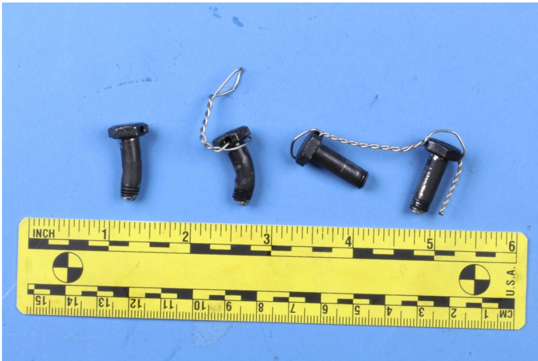
Figure 1: Crankshaft gear bolts.
