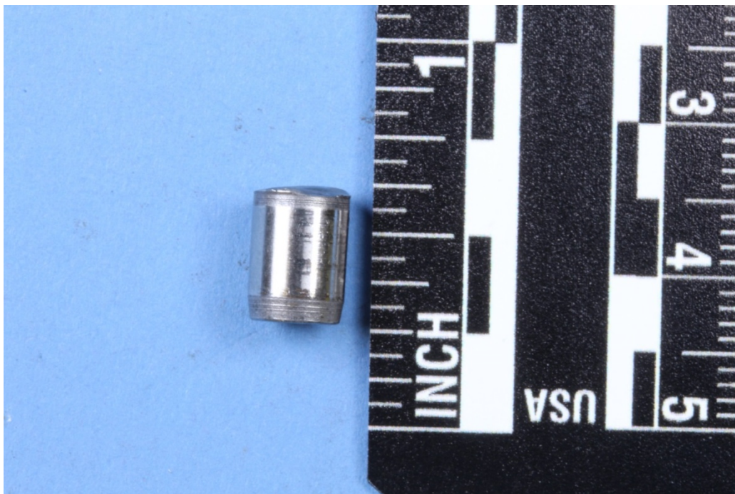
Figure 4: Portion of the crankshaft gear dowel pin.
