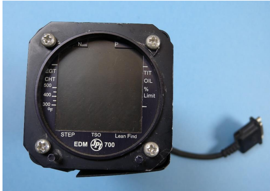
Figure 1. Damaged exterior of device, front view.
