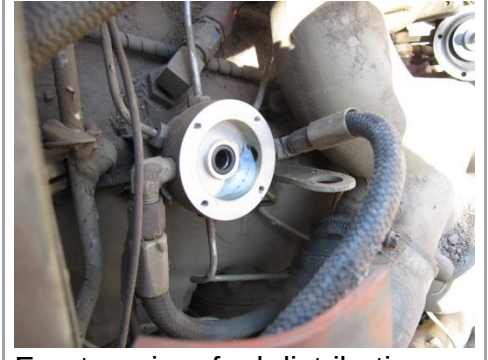
Front engine, fuel distribution valve showing fuel present.
