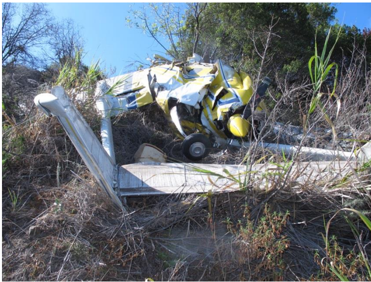
Tail section with left and right tail booms.
