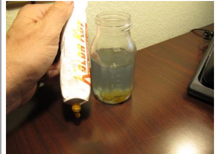
Front engine fuel water test.
