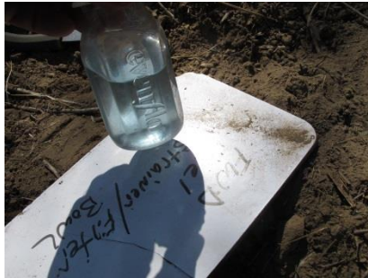
Fuel drained from front engine bowl.
