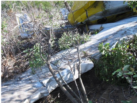
Inboard section of the right wing.
