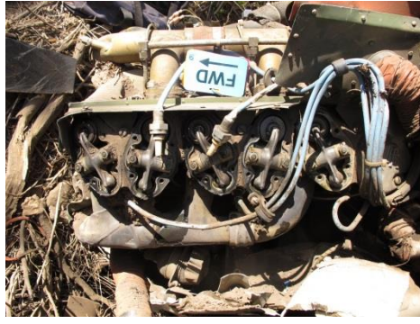
Front engine, right side with valve covers removed.
