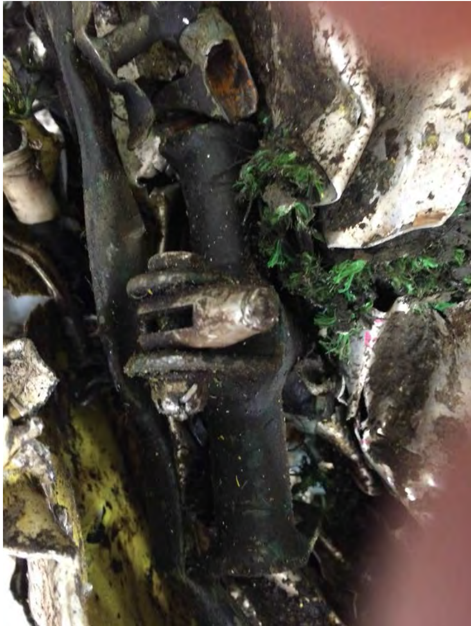
Figure 5 Elevator Push-Pull Tube Rod End at T-bar
