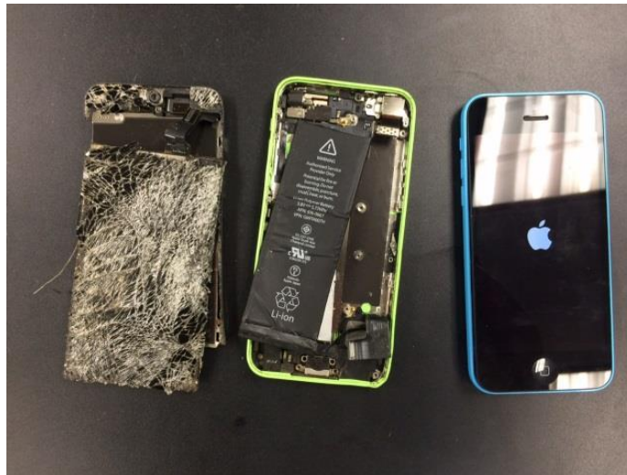
Figure 4. The NTSB surrogate device (right) booting with the accident device's circuitry installed.
