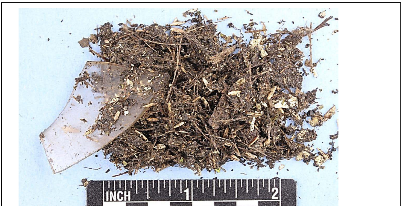
Figure 5. As-received grease sample from the engine cooling fan.
