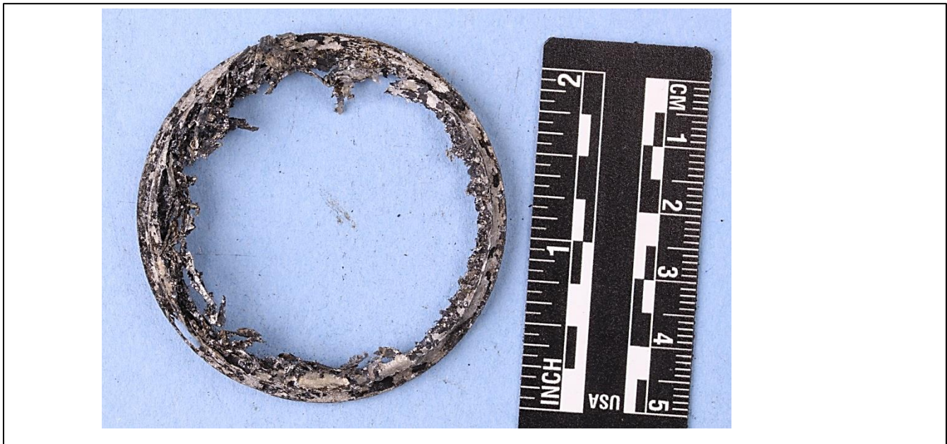
Figure 4. Remains of the plug (bump stop) Lycoming P/N 77416, which fits between the drive adapter and the engine crankshaft flange.
