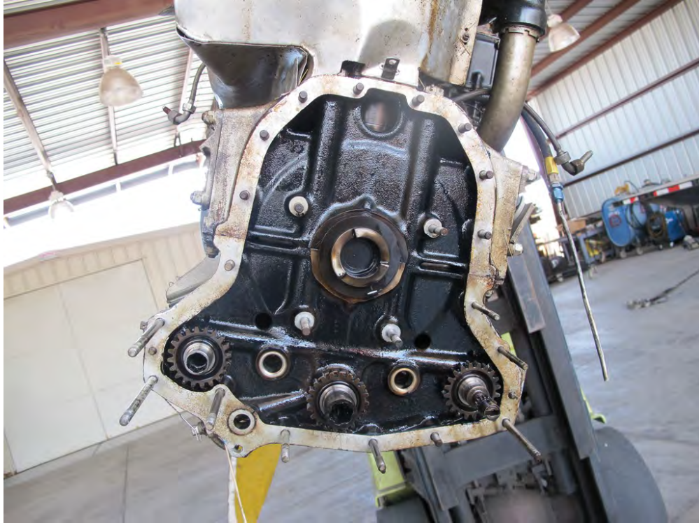
Photo 21 Back of Engine with Accessory Case Removed
