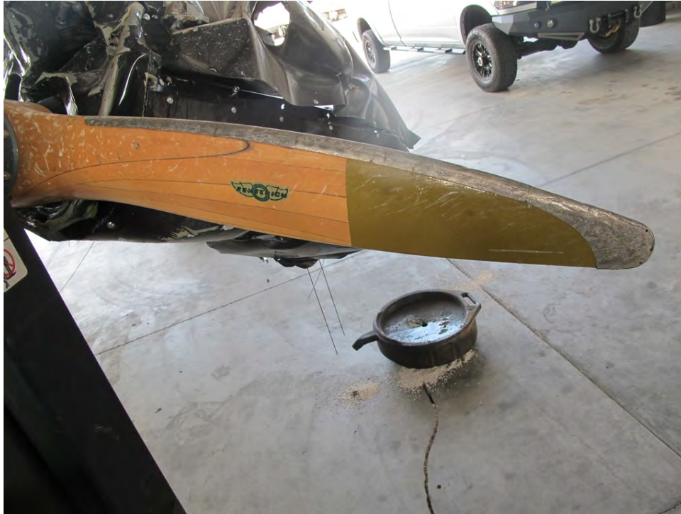
Photo 28 Intact Propeller Blade
