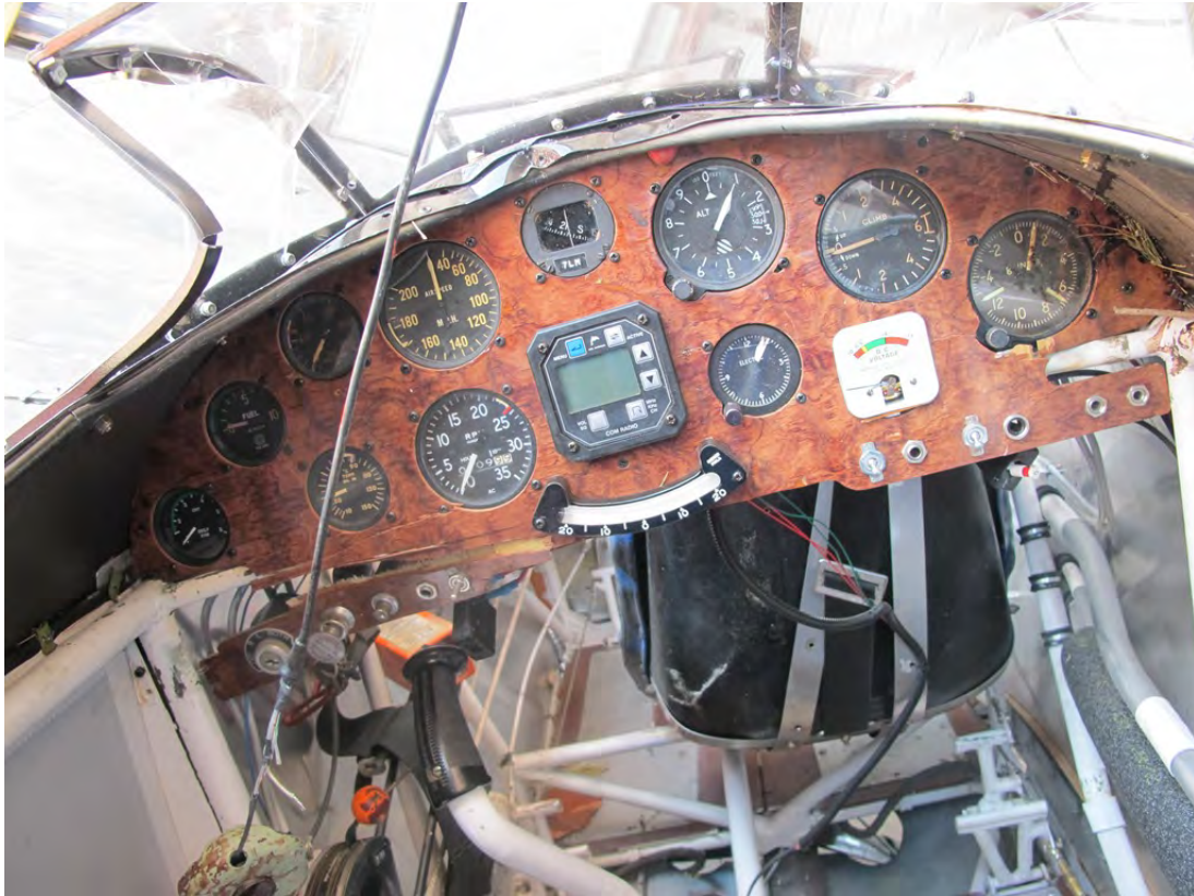
Photo 3 Rear Instrument Panel
