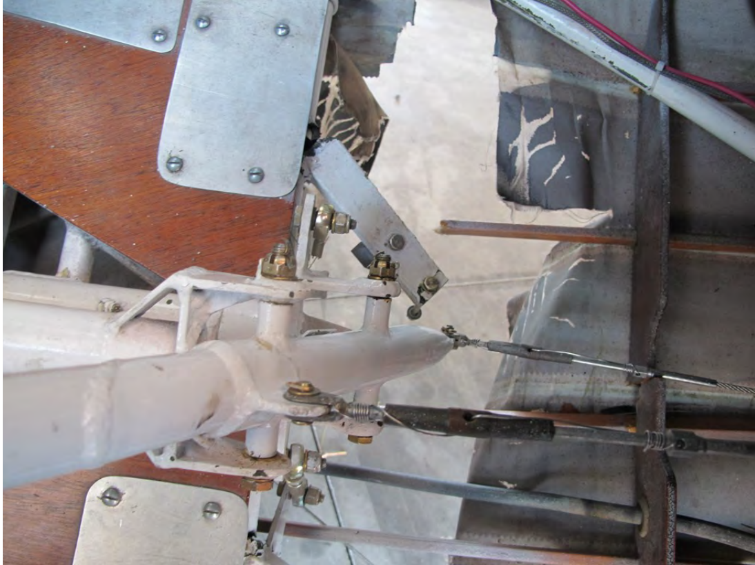
Photo 2 Rear Yoke Flight Control Connections
