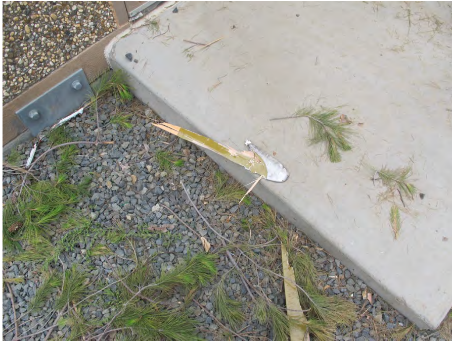
Photo 13 Separated Blade Tip
