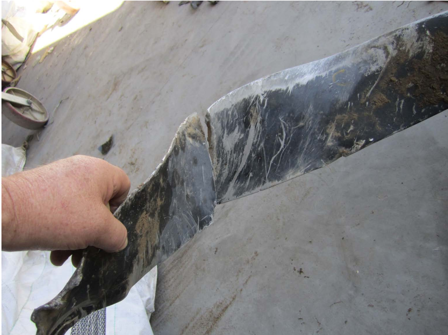
ASI-15-AF-118 Propeller blade separation
