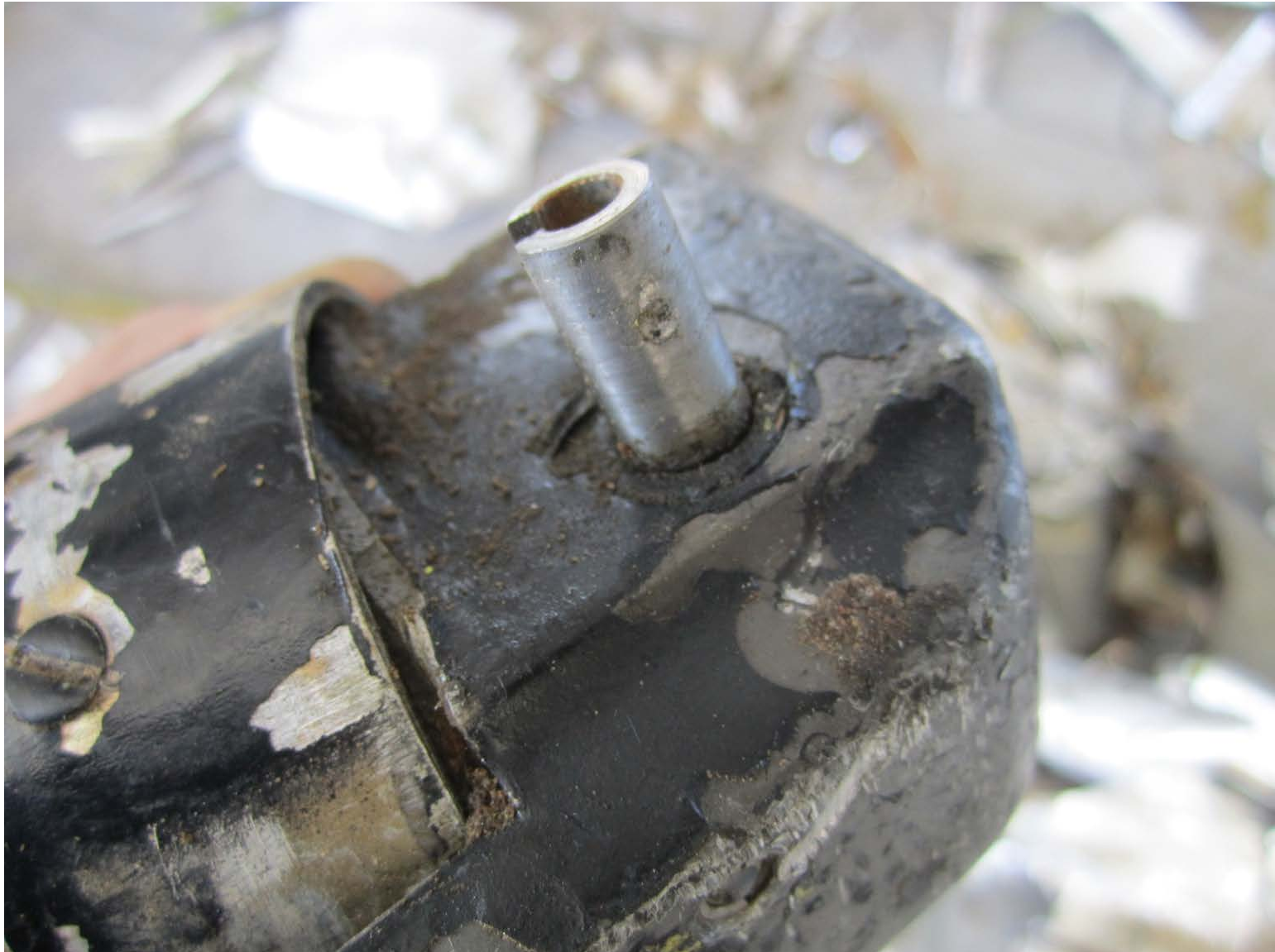
ASI-15-AF-085 Flap drive showing collar screw indent
