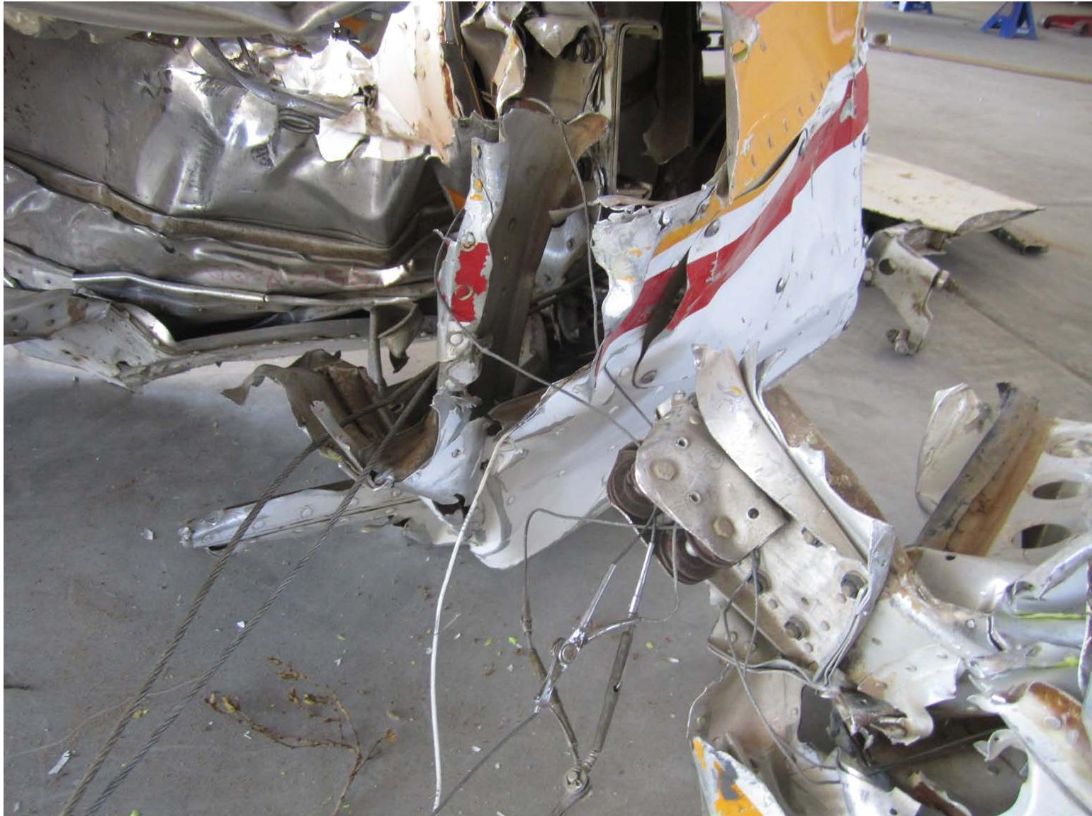
ASI-15-AF-110 Pitch, yaw, and trim cables in rear fuselage
