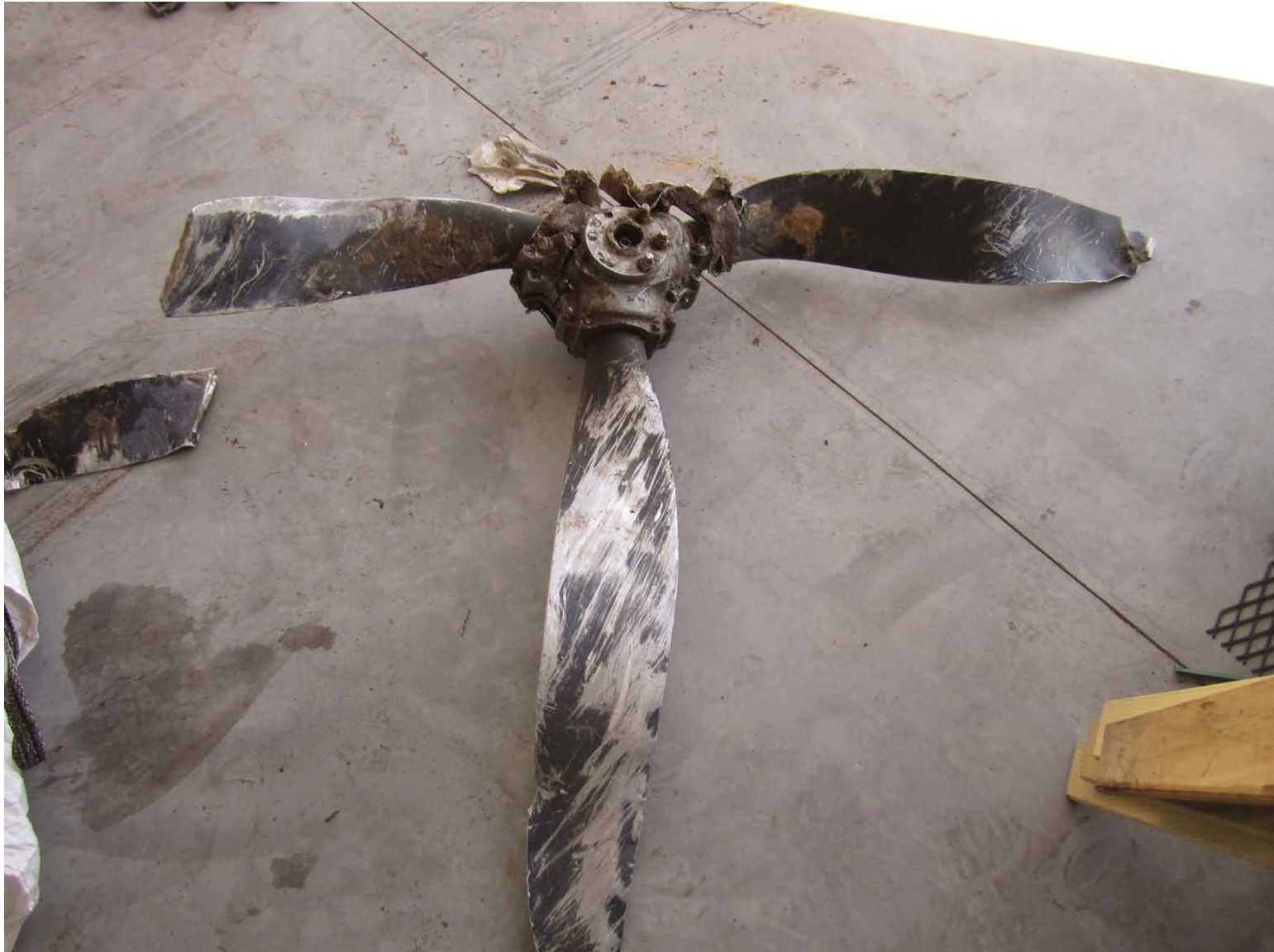
ASI-15-AF-117 Propeller showing blade faces
