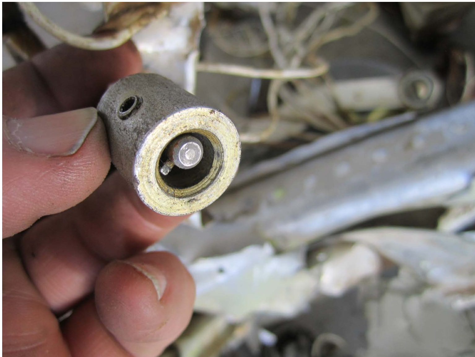
ASI-15-AF-087 Flap collar and key on flap cable
