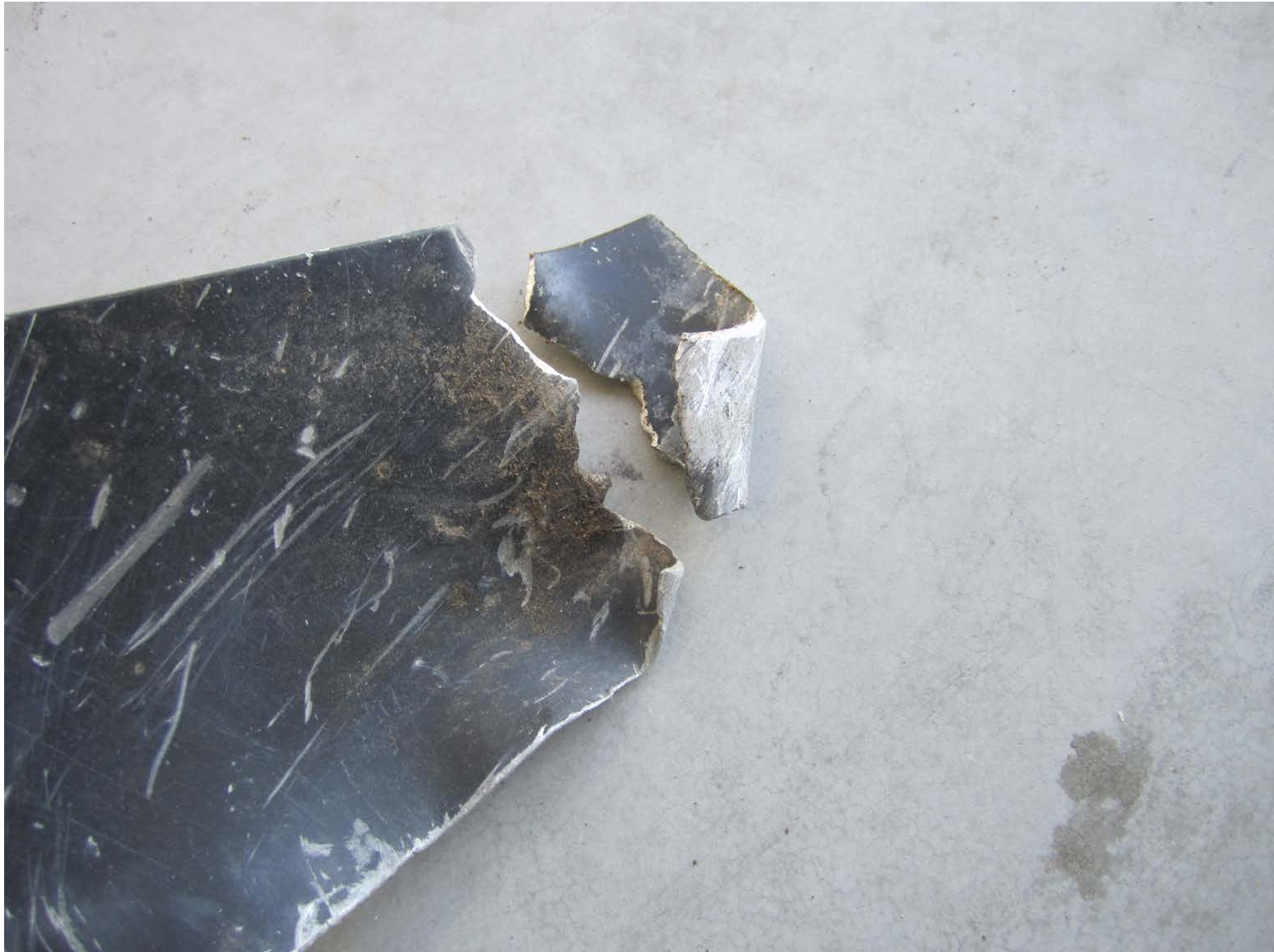
ASI-15-AF-121 A blade tip separated
