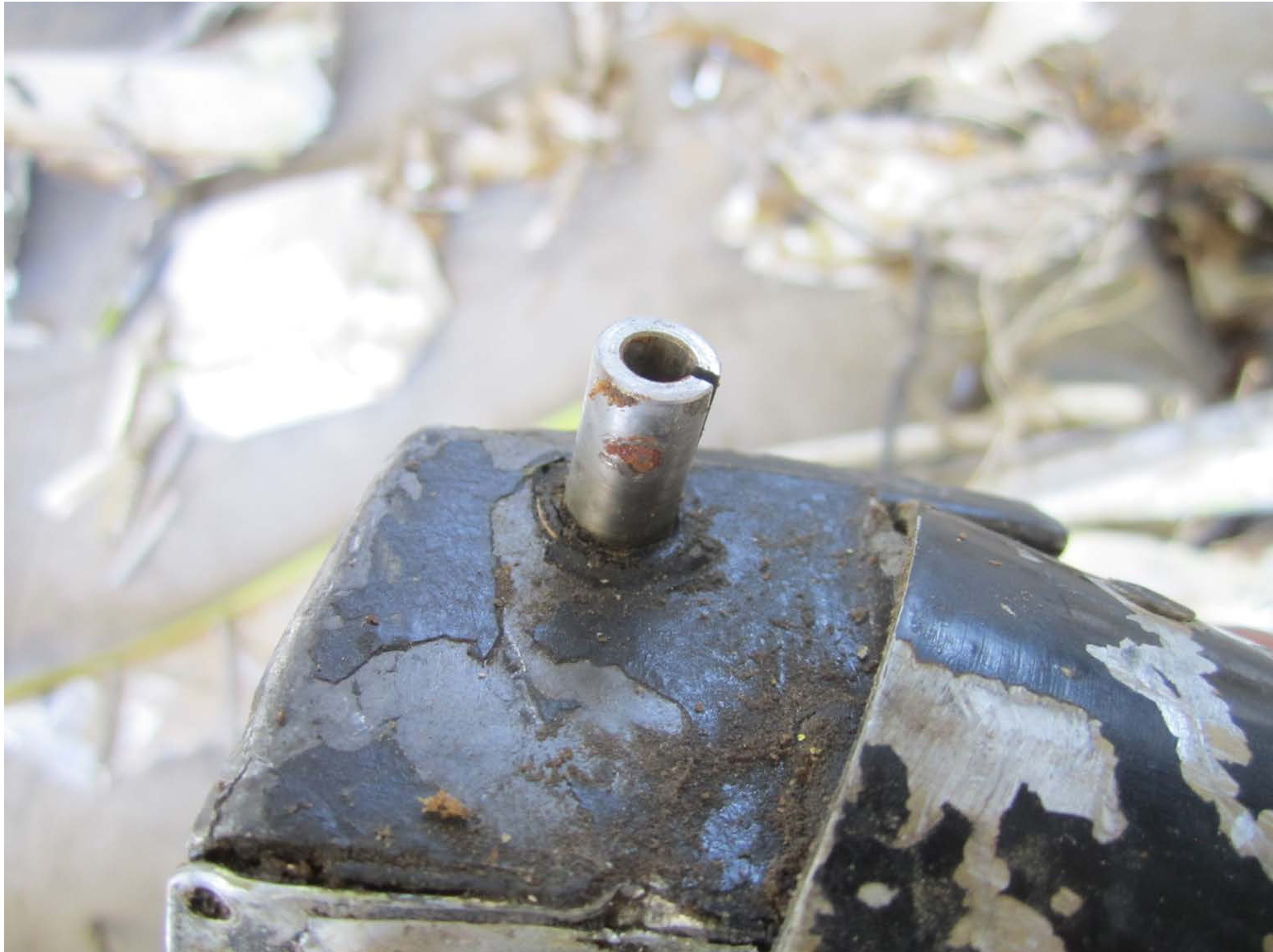
ASI-15-AF-086 Flap drive showing collar screw indent
