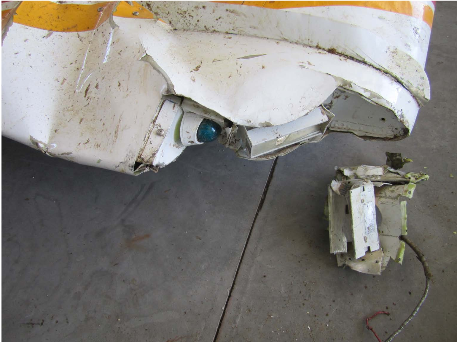
ASI-15-AF-114 Right wing nav light and left wing strobe light box
