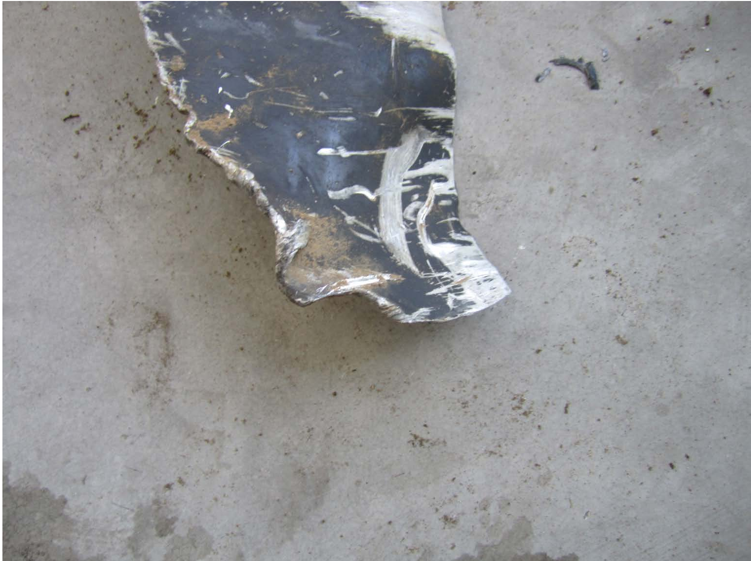
ASI-15-AF-119 A blade tip separation
