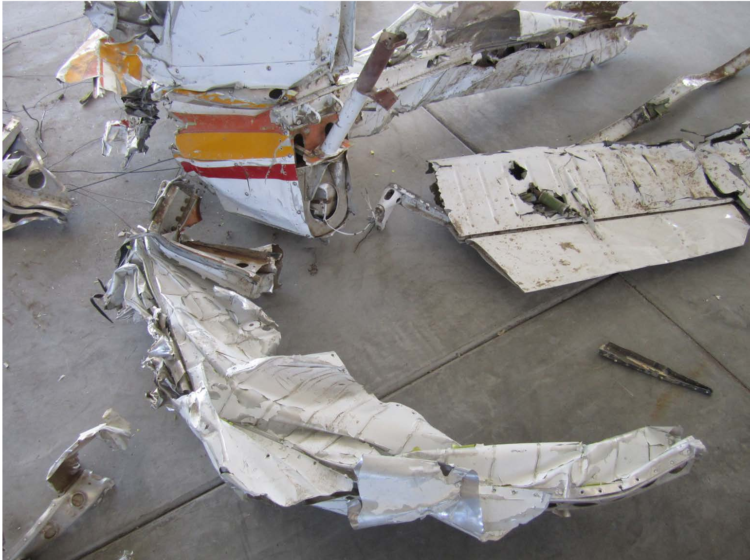
ASI-15-AF-113 Angle at which left horizontal stabilizer deformed
