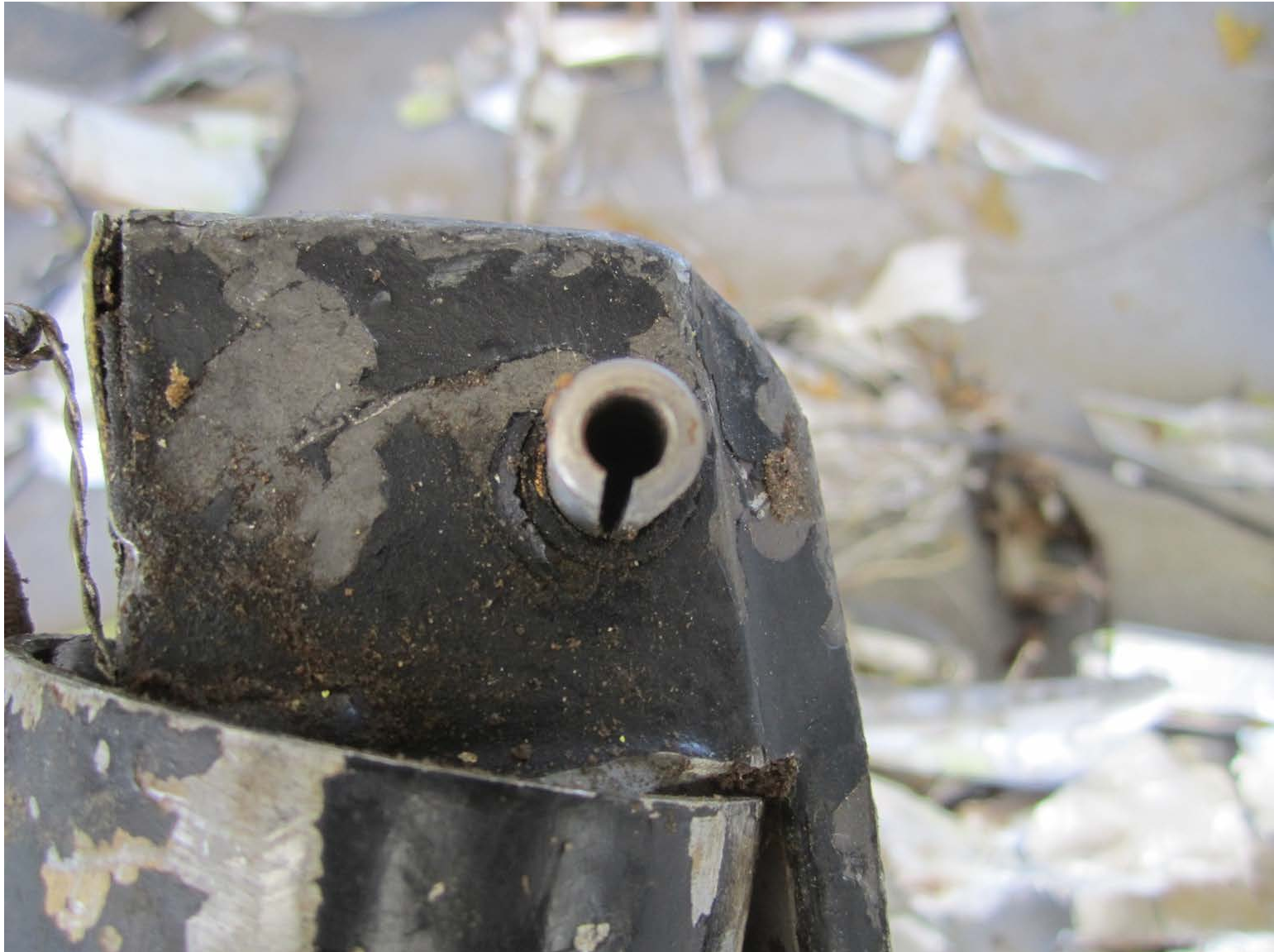
ASI-15-AF-084 Flap drive showing key slot
