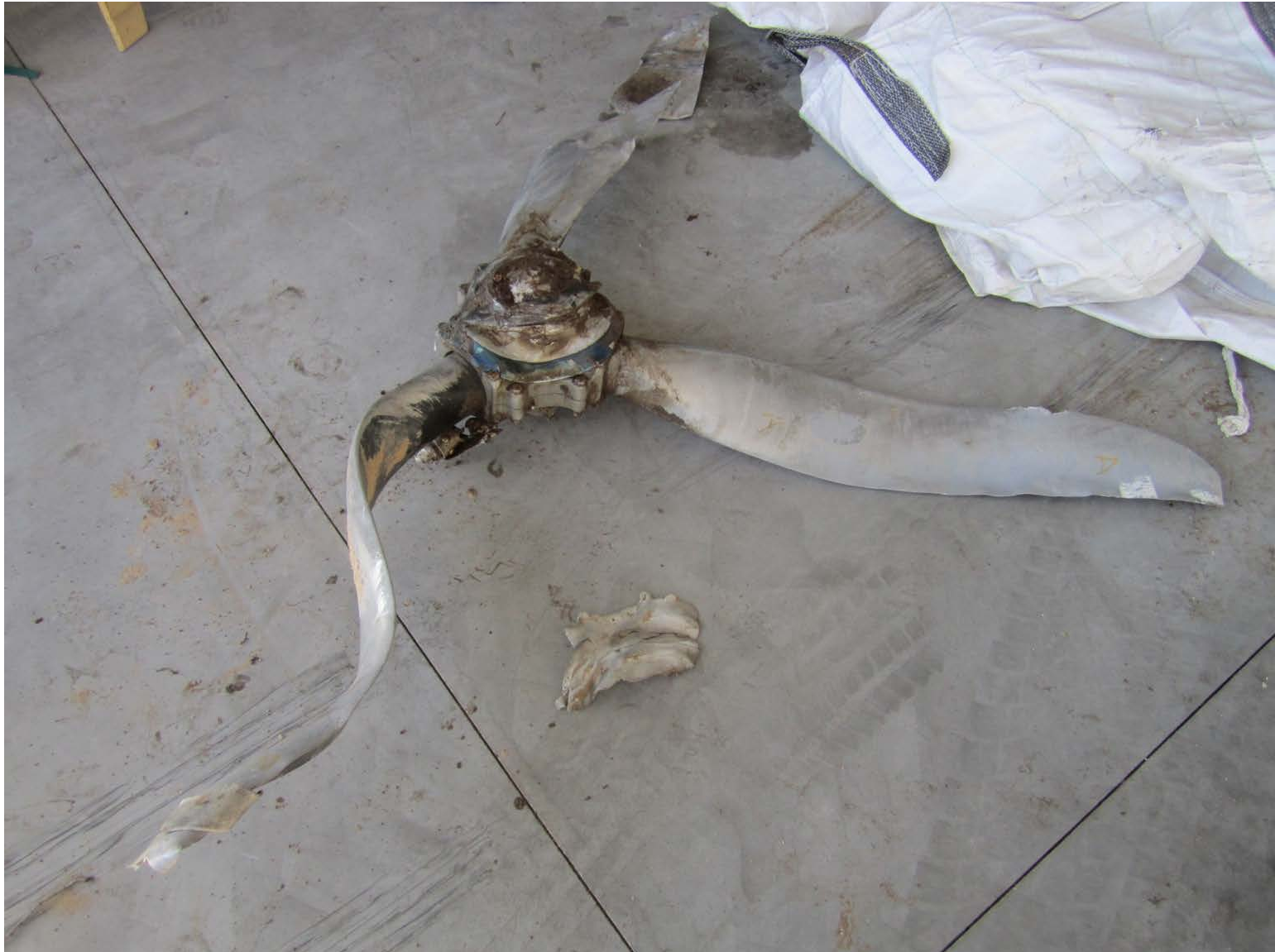
ASI-15-AF-123 Propeller blade showing blade backs
