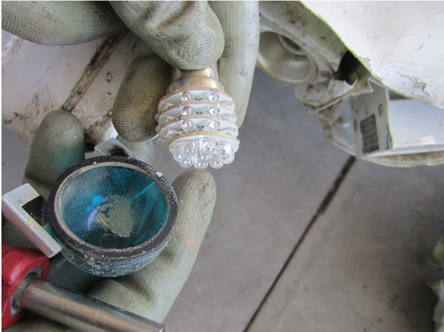
ASI-15-AF-115 Right nav light bulb – LED light
