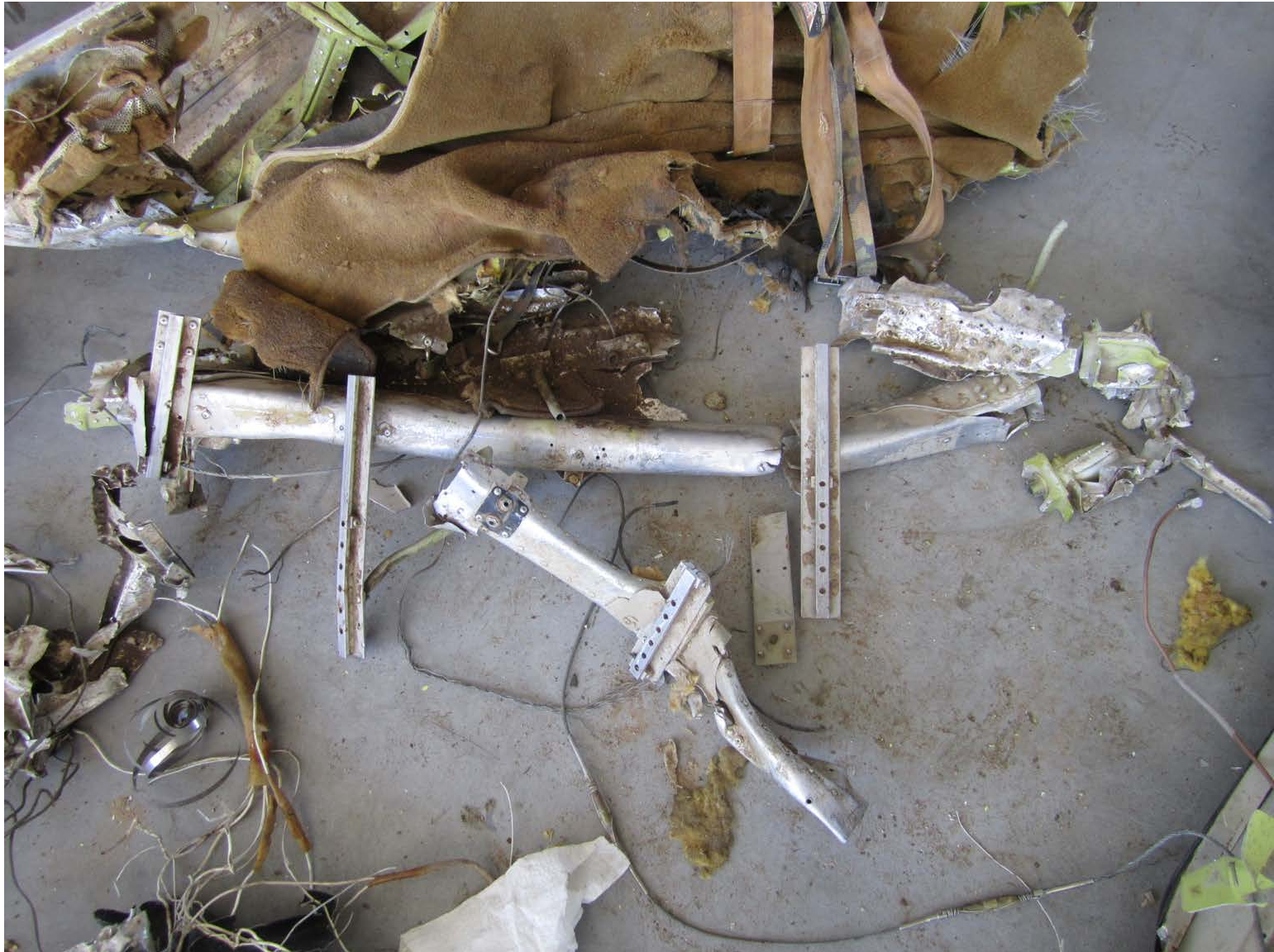
ASI-15-AF-091 Rear carry through structure showing seat tracks
