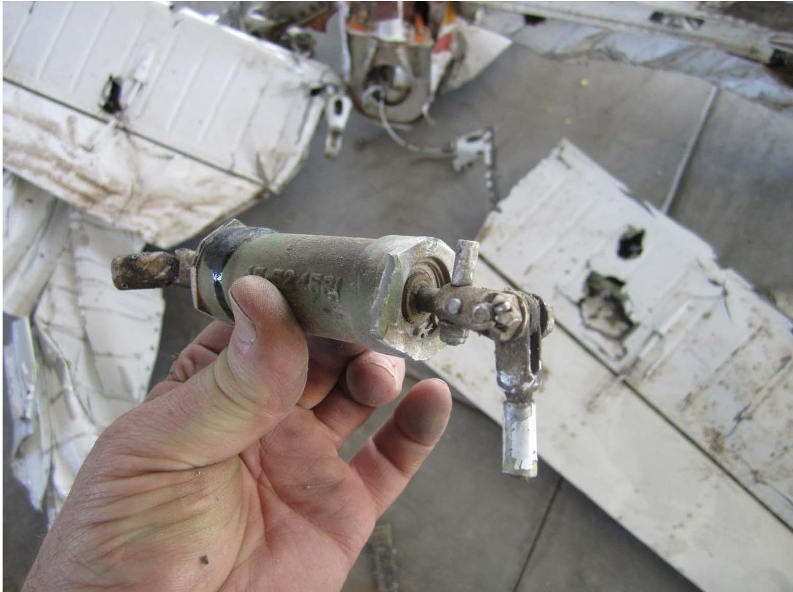
ASI-15-AF-112 Right (black) elevator trim tab actuator (retracted)
