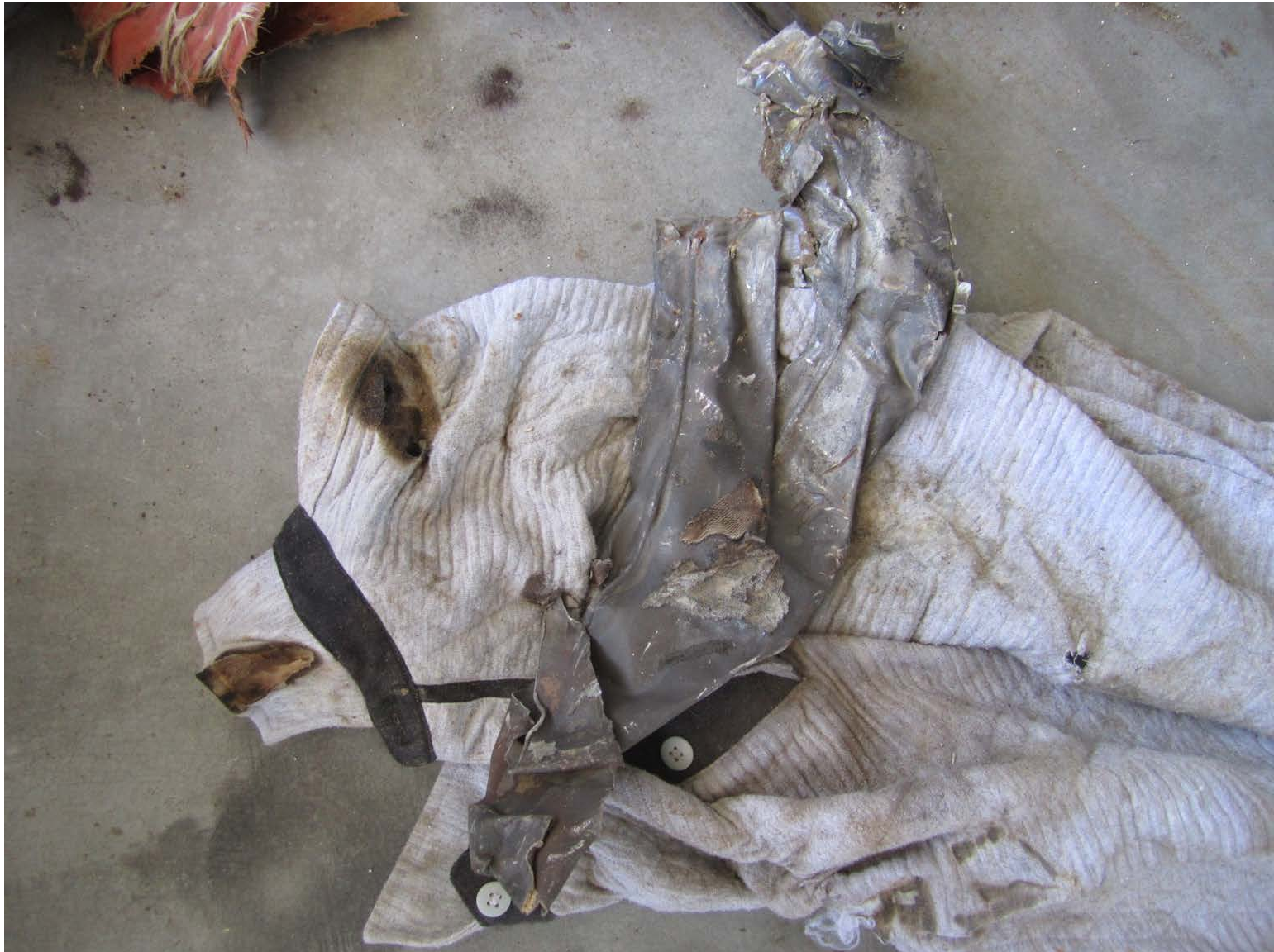
ASI-15-AF-127 A clothing article was found melted to a muffler
