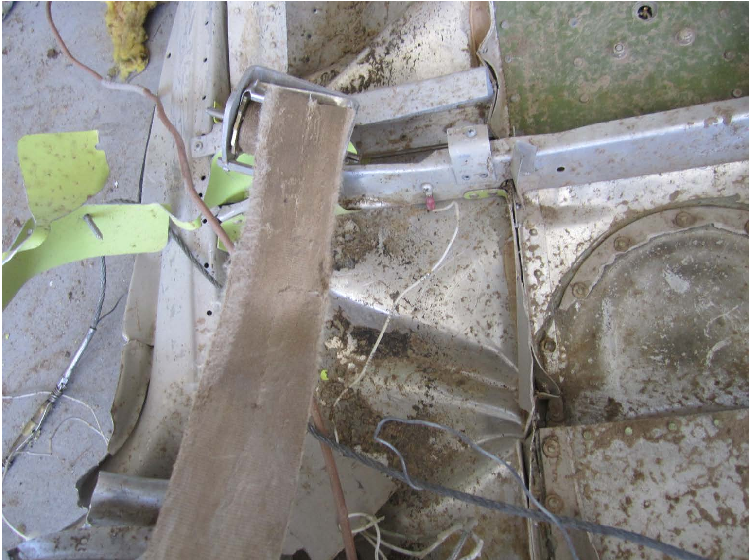
ASI-15-AF-104 A pilot shoulder belt showing stretching
