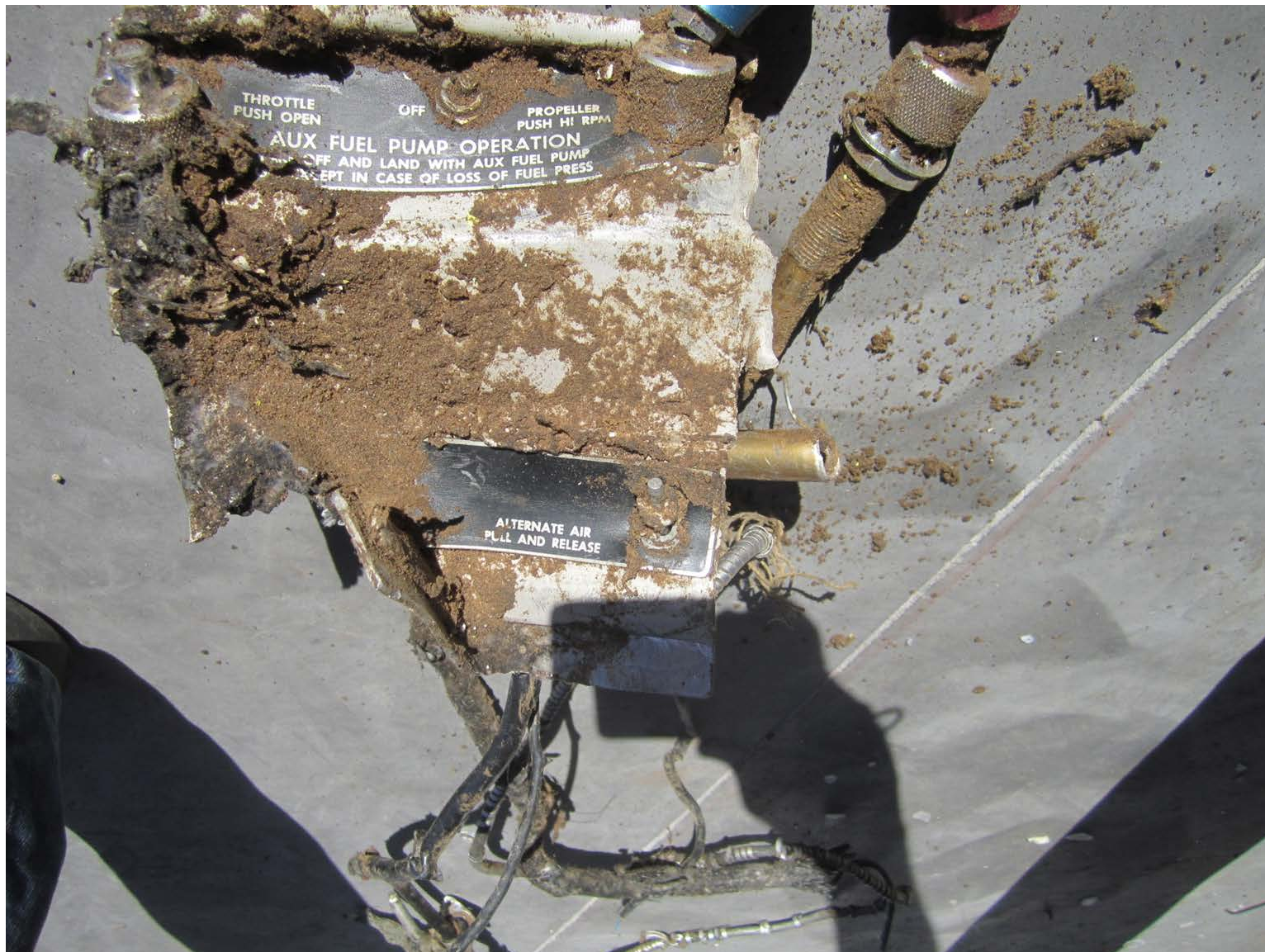
ASI-15-AF-129 Engine controls, placard, and fuel boost pump switch
