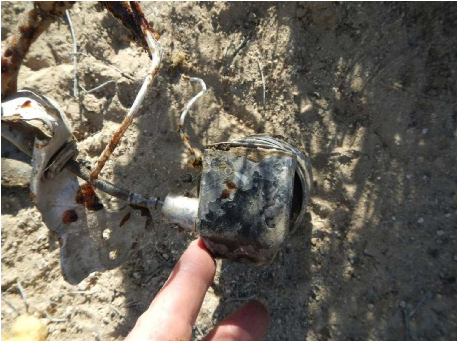
ASI-15-AF-20 Flap cable/housing and flap drive assembly
