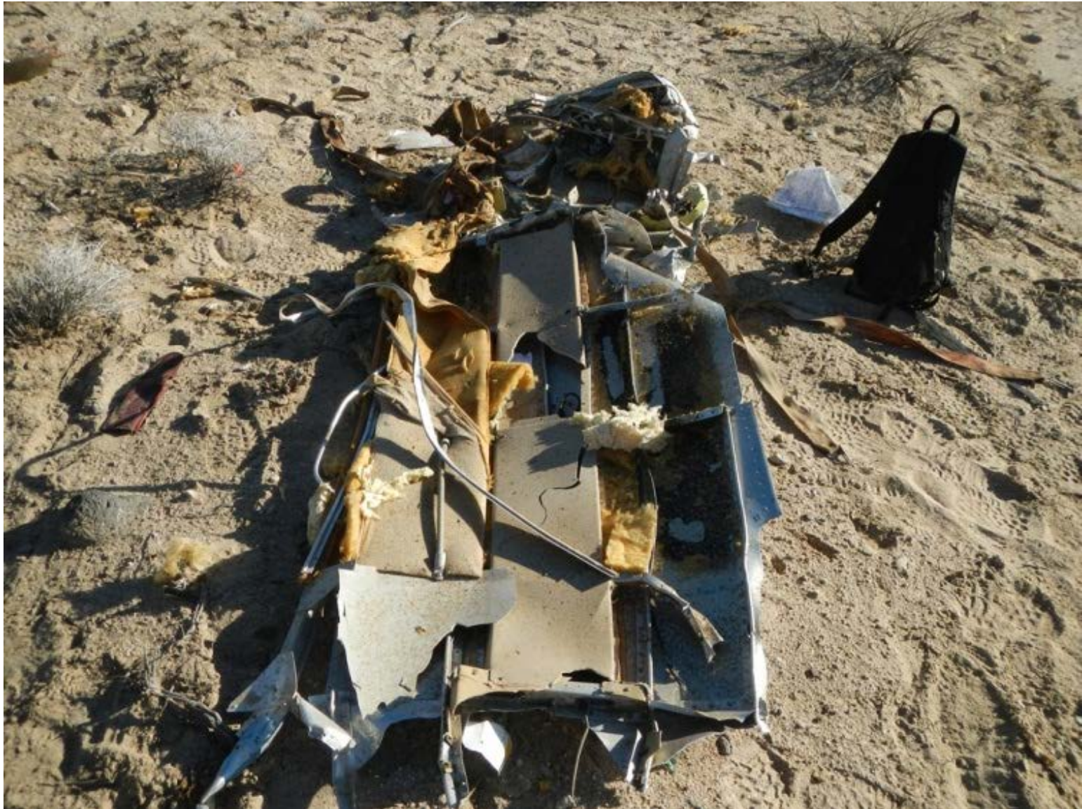
ASI-15-AF-41 Cabin roof interior
