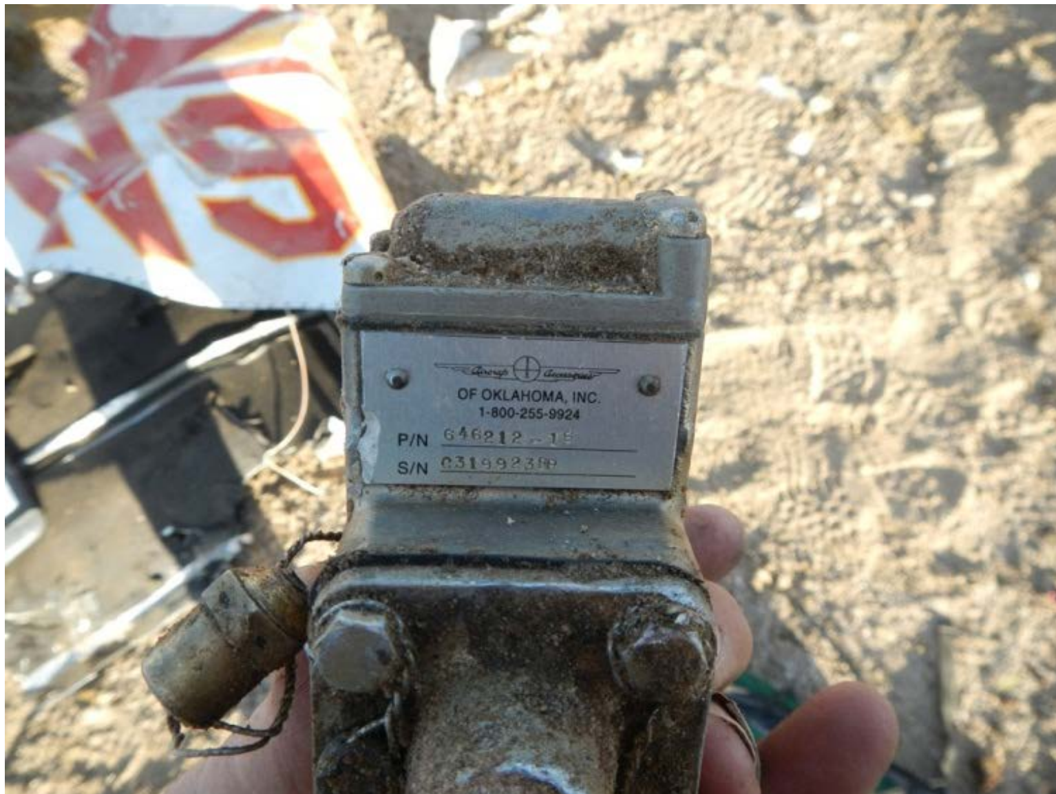
ASI-15-AF-67 Engine driven fuel pump and identification plate
