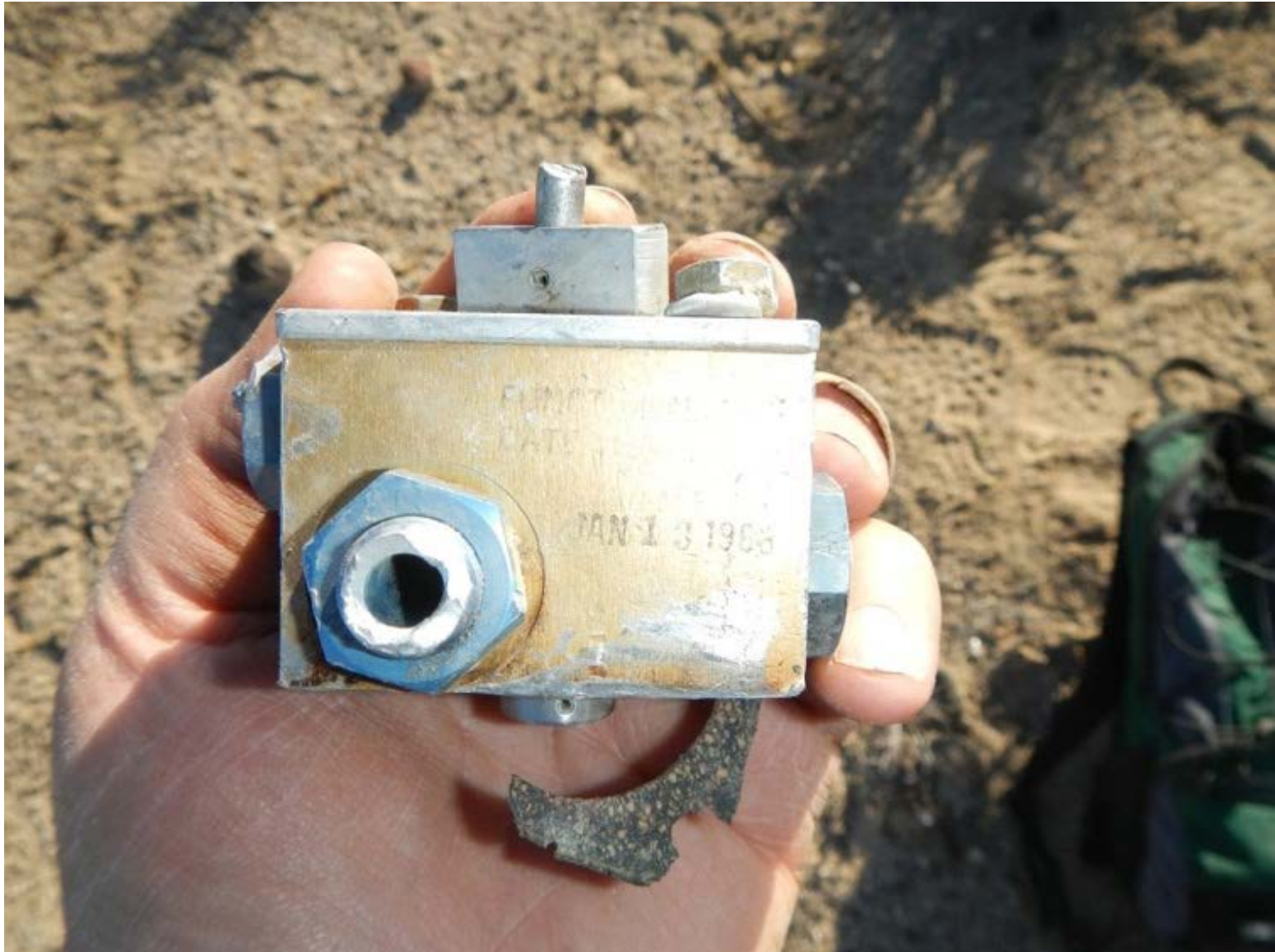
ASI-15-AF-56 Selector valve left wing tank input
