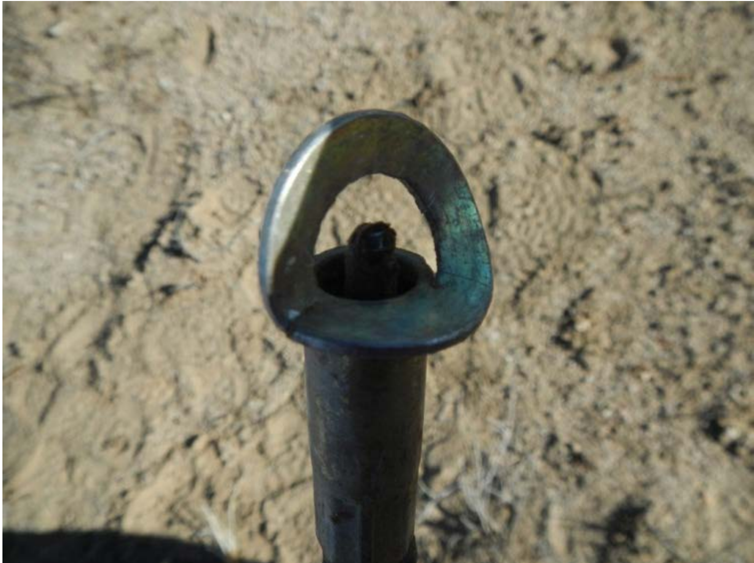
ASI-15-AF-22 Flap drive actuator end showing cable key
