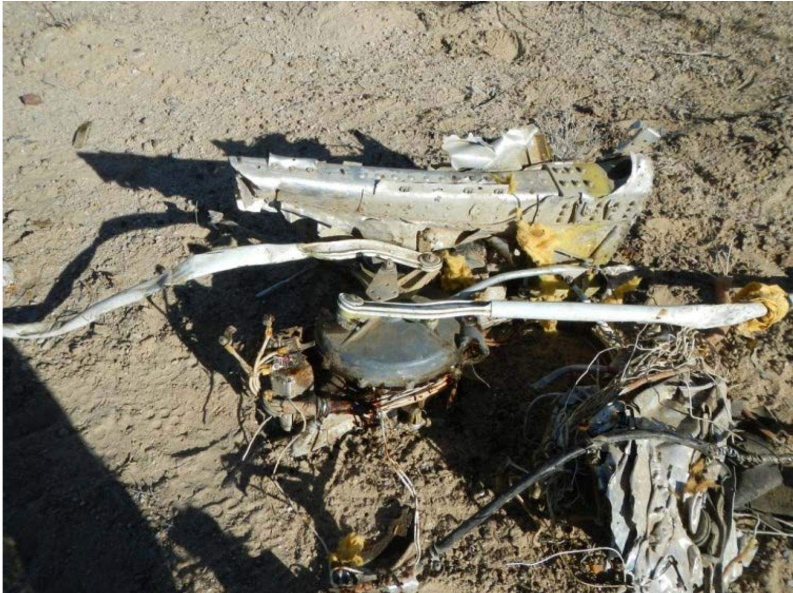
ASI-15-AF-18 Landing gear actuator and section of front carry through
