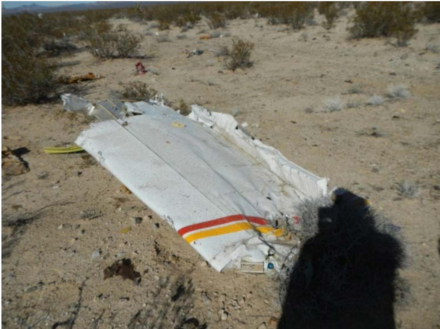
ASI-15-AF-13 Right outboard wing and aileron
