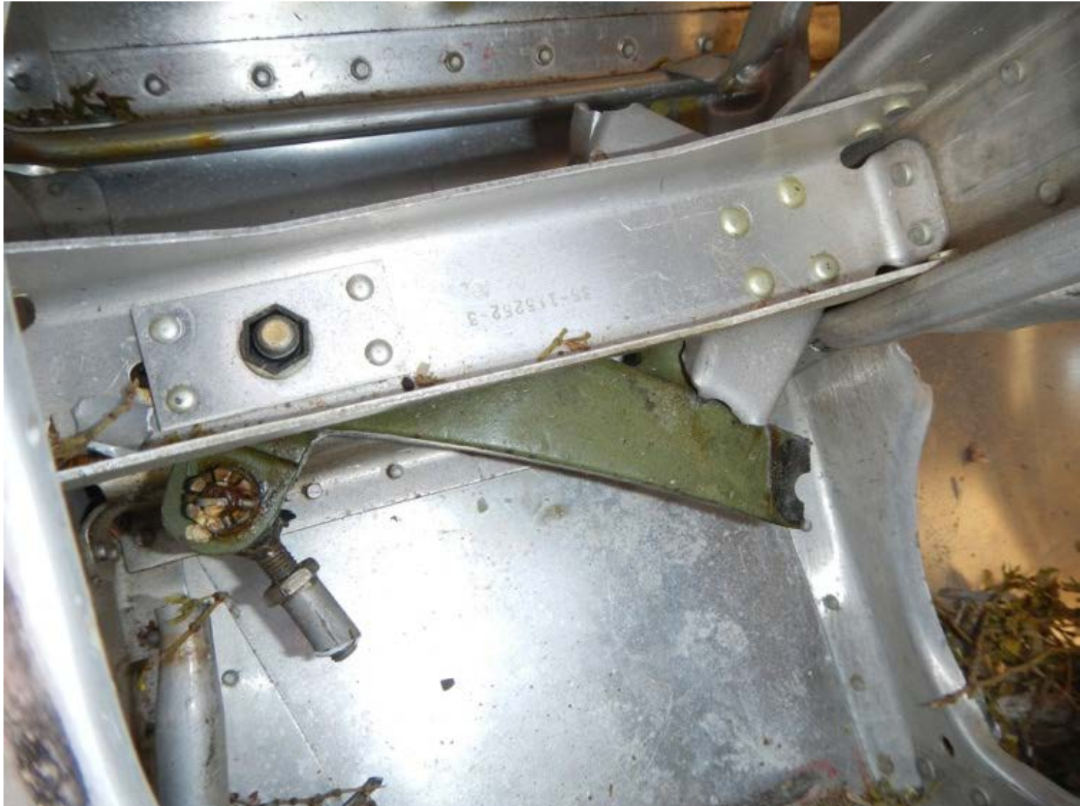
ASI-15-AF-69 Right aileron bell crank and pushrod
