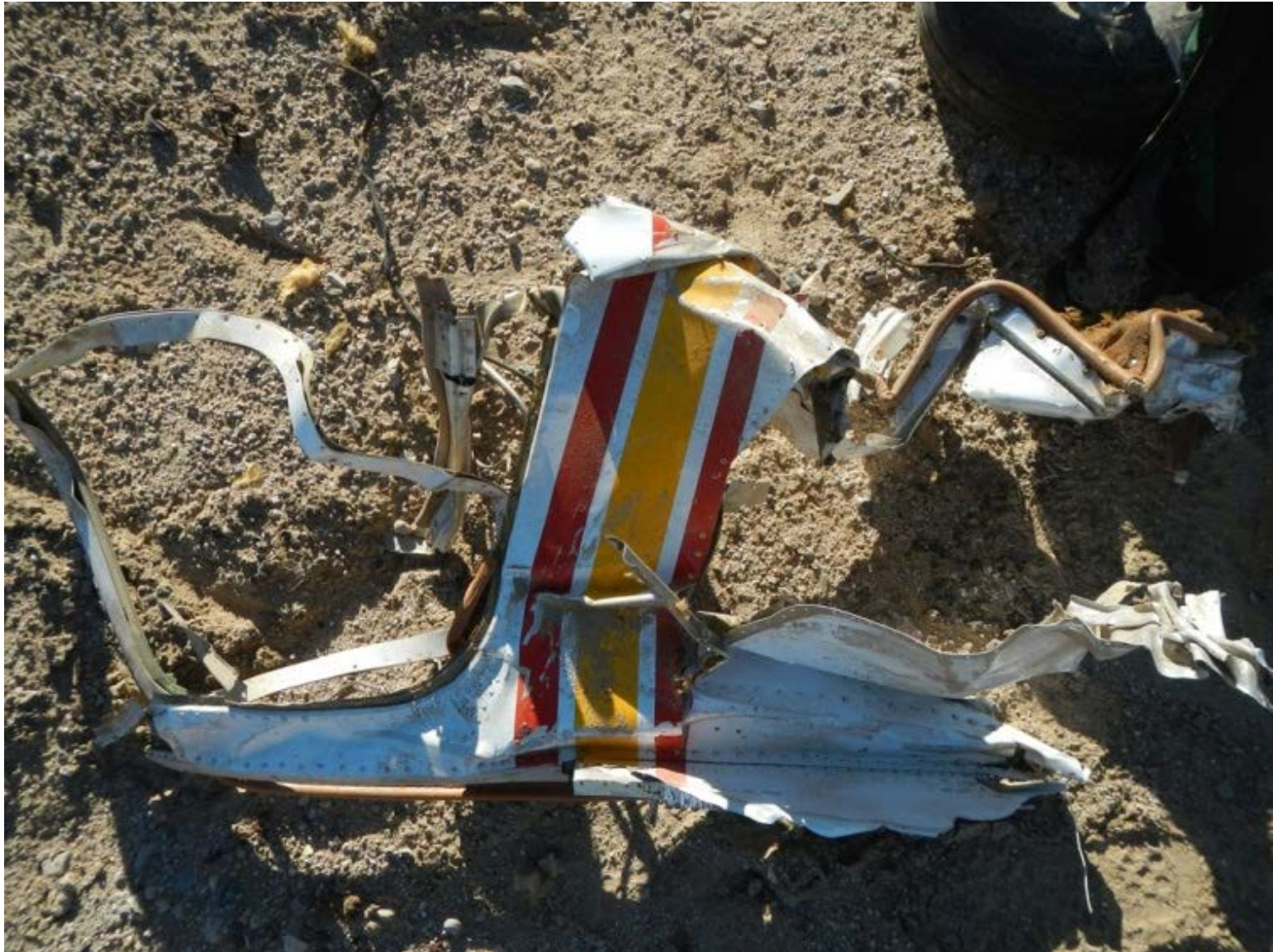
ASI-15-AF-40 Right fuselage between doors emergency exit
