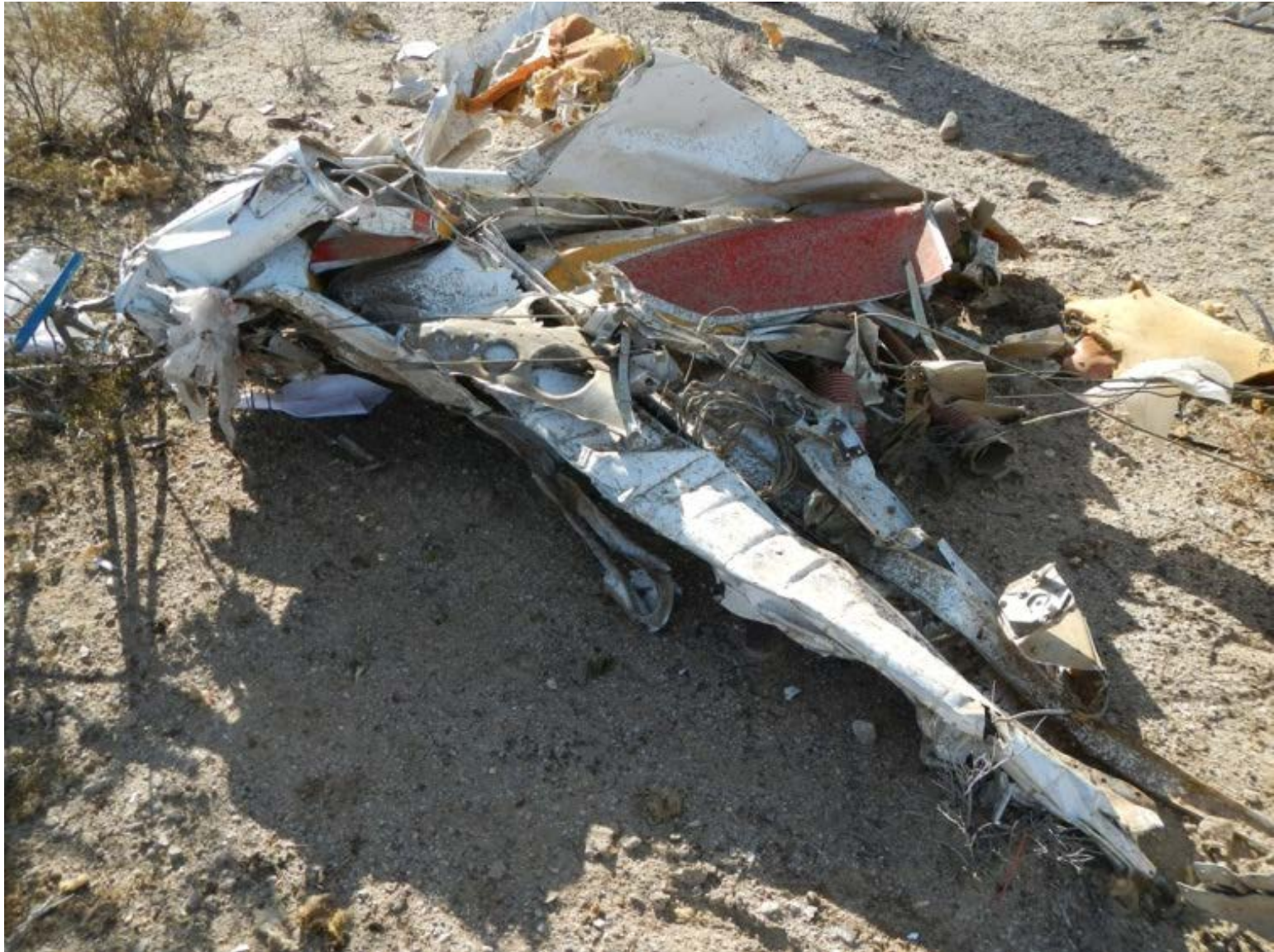
ASI-15-AF-12 Rear fuselage and empennage surfaces
