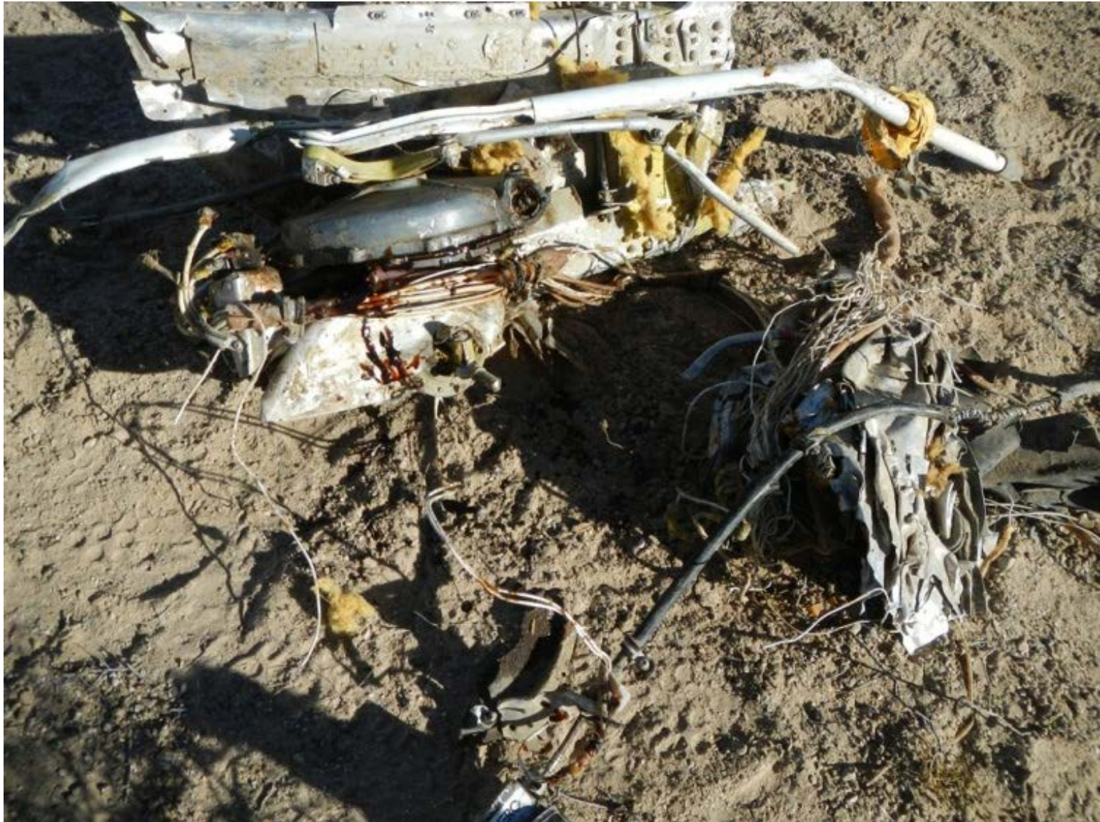
ASI-15-AF-19 Landing gear actuator and section of front carry through
