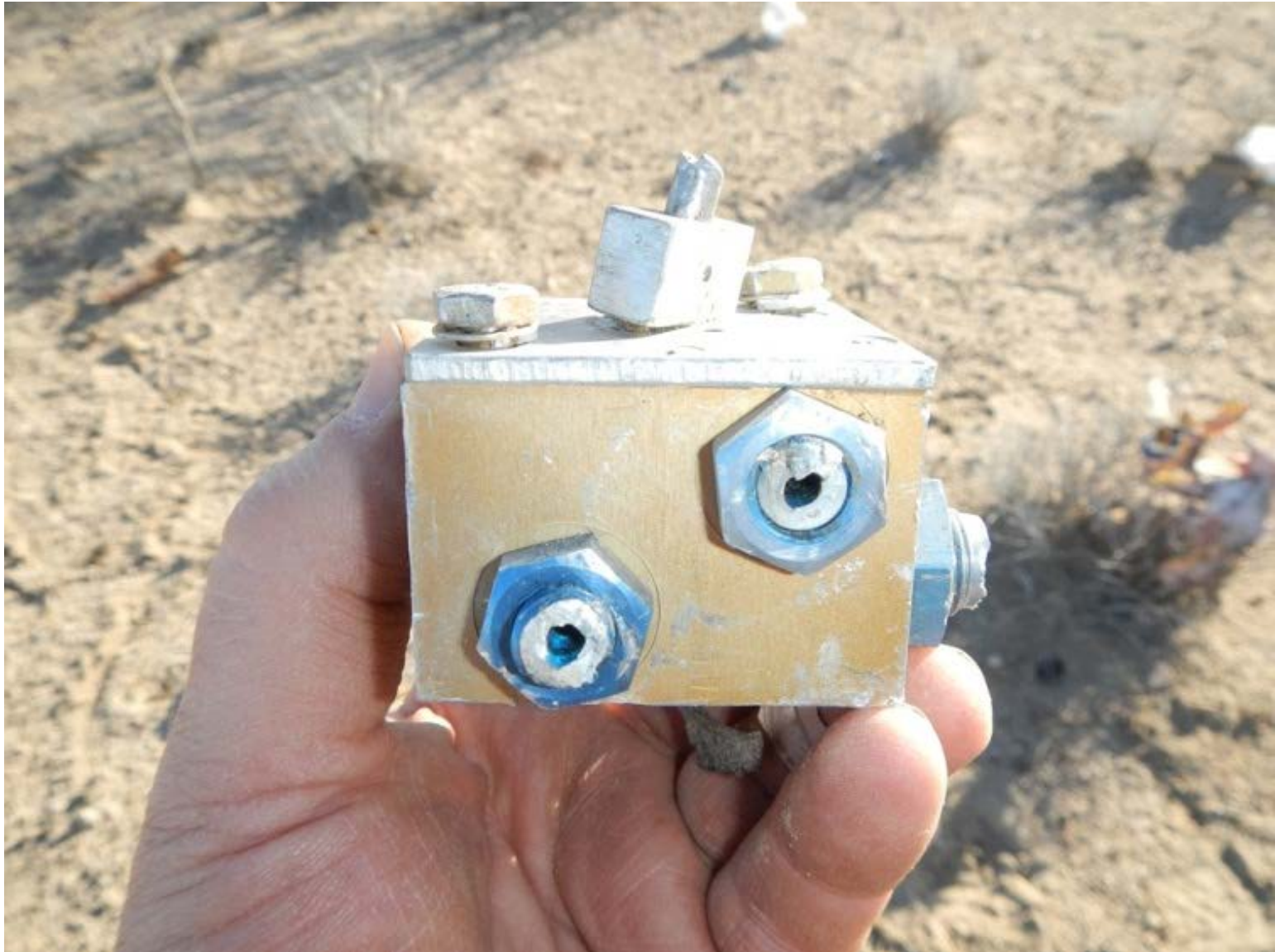
ASI-15-AF-53 Fuel selector valve return lines
