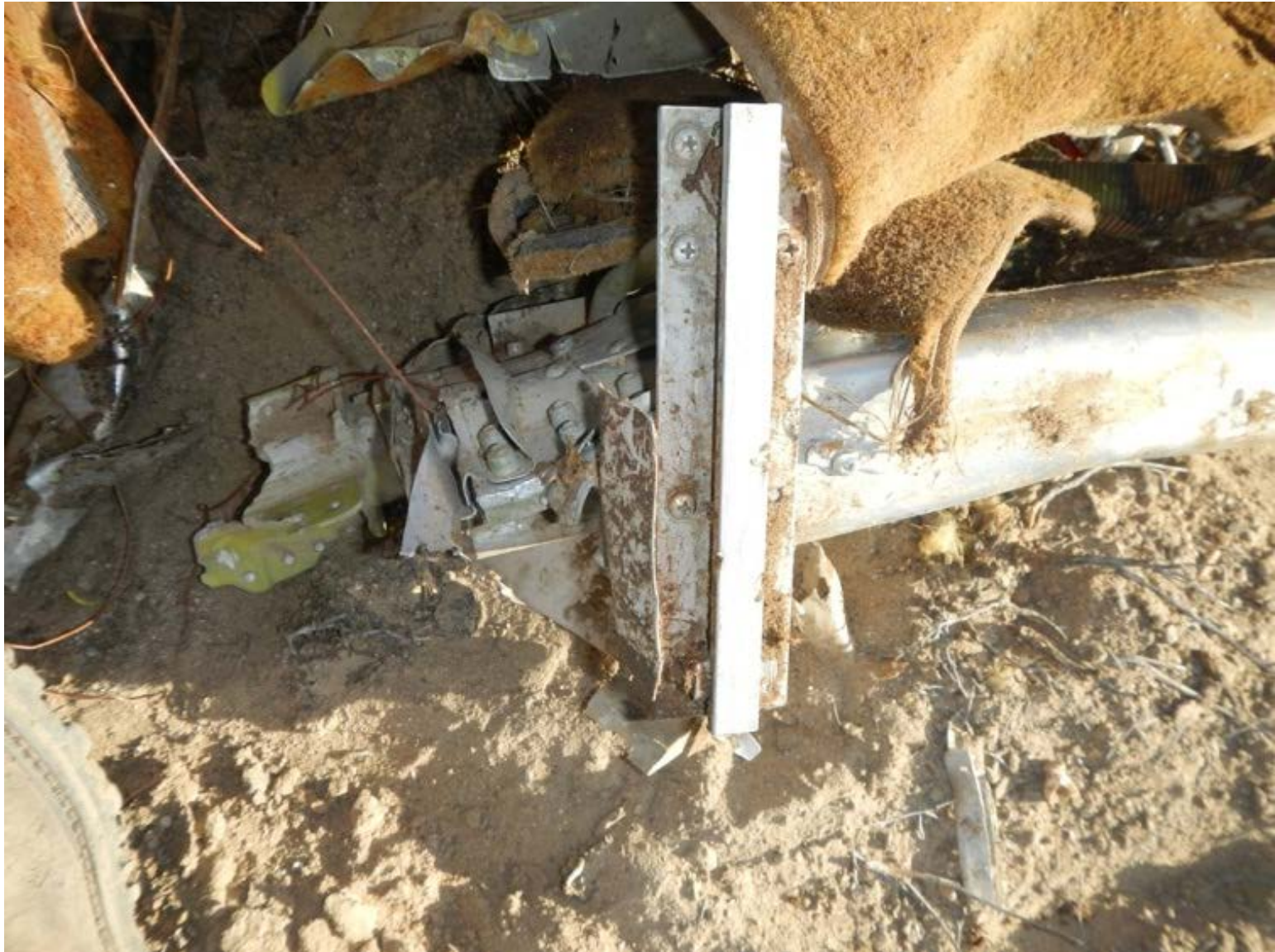
ASI-15-AF-60 Front carry through, right side showing wing attach fitting and seat track
