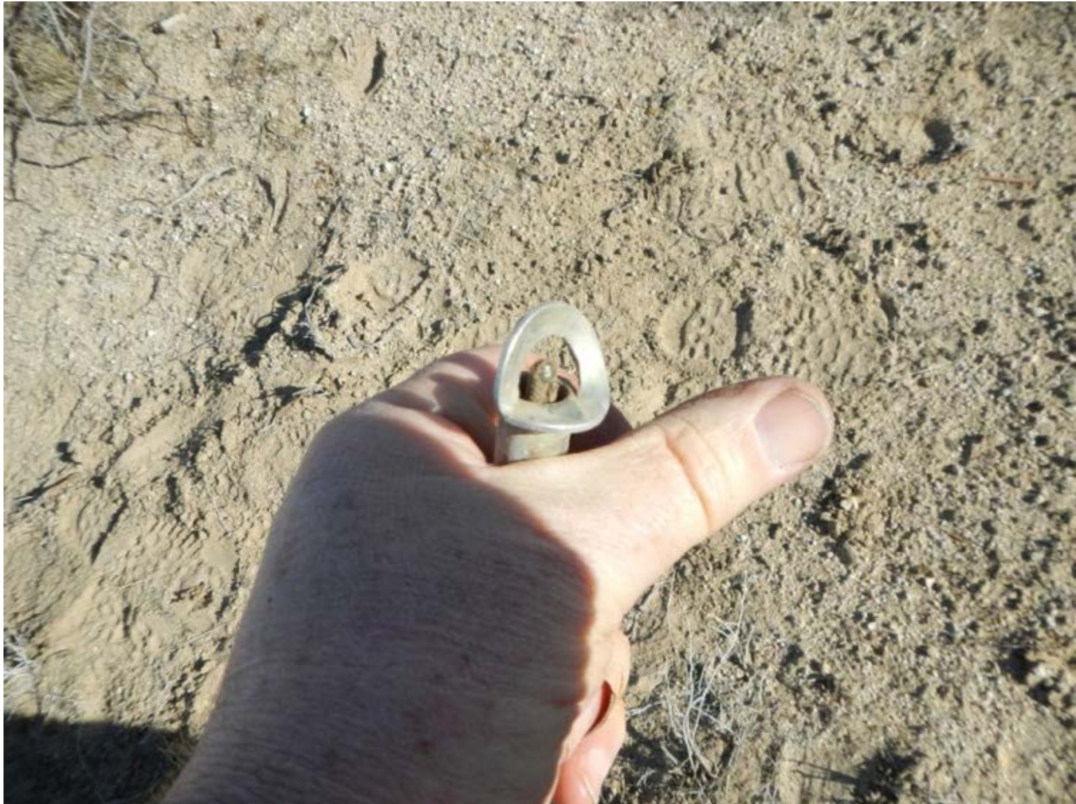
ASI-15-AF-23 Flap drive actuator end showing cable key
