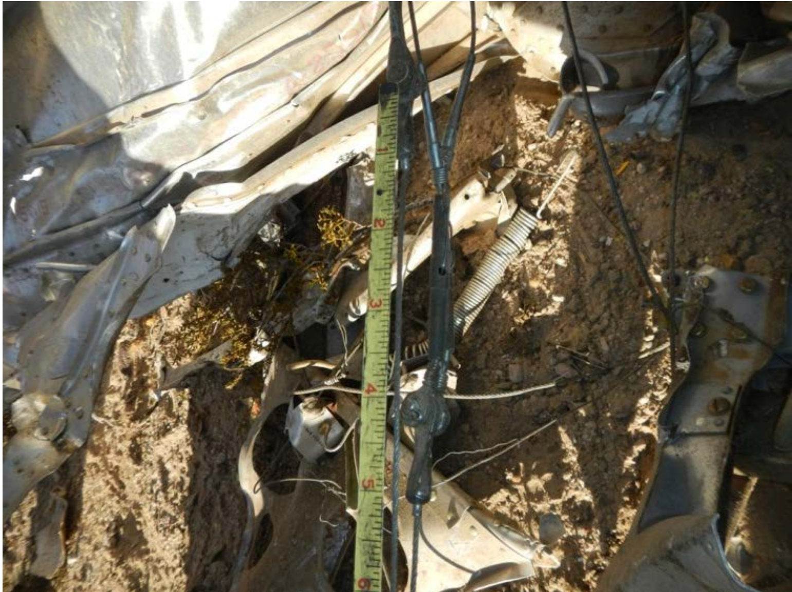
ASI-15-AF-57 Pitch trim cables; difference between UP/DOWN cable ends
