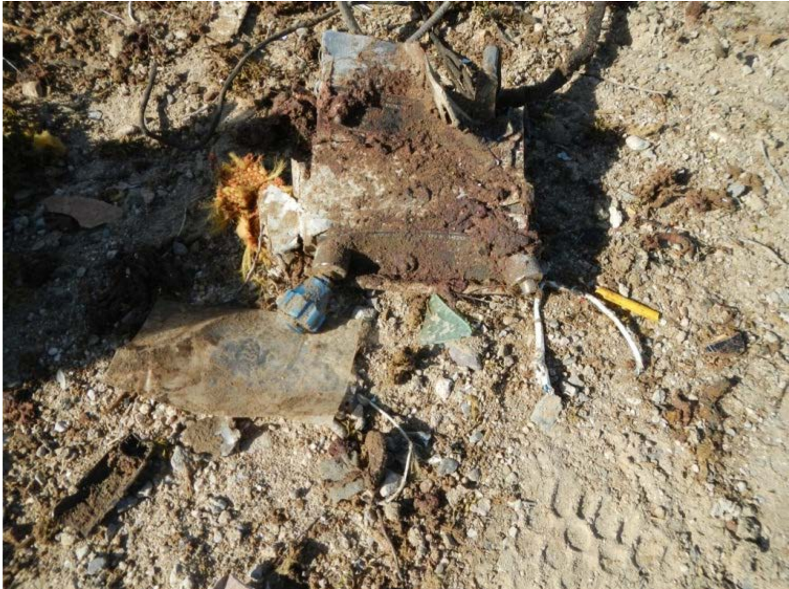
ASI-15-AF-07 Engine control panel
