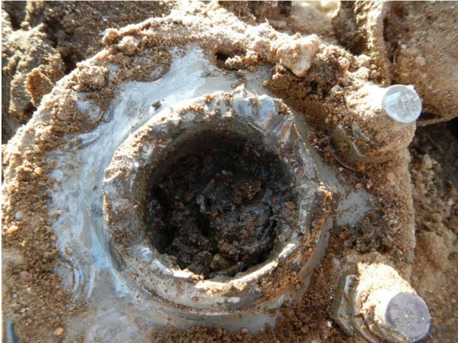
ASI-15-AF-82 Engine crankshaft separation at the propeller flange
