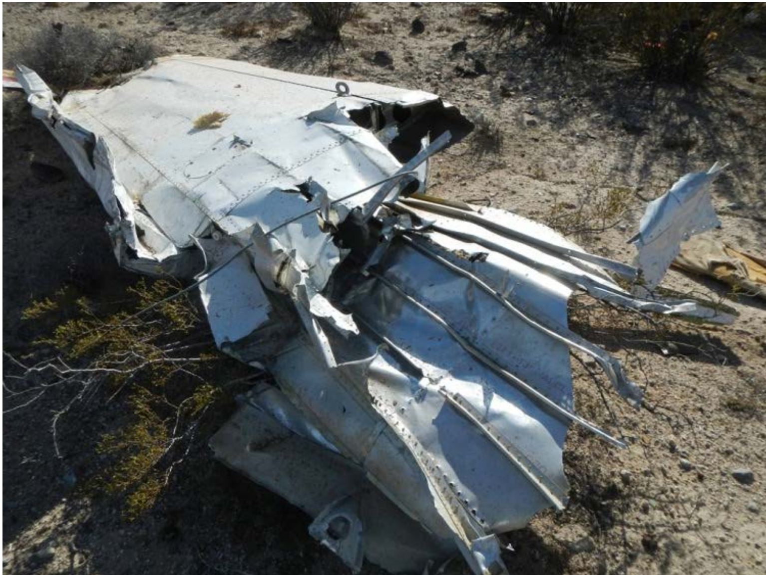
ASI-15-AF-15 Bottom side of right outboard wing
