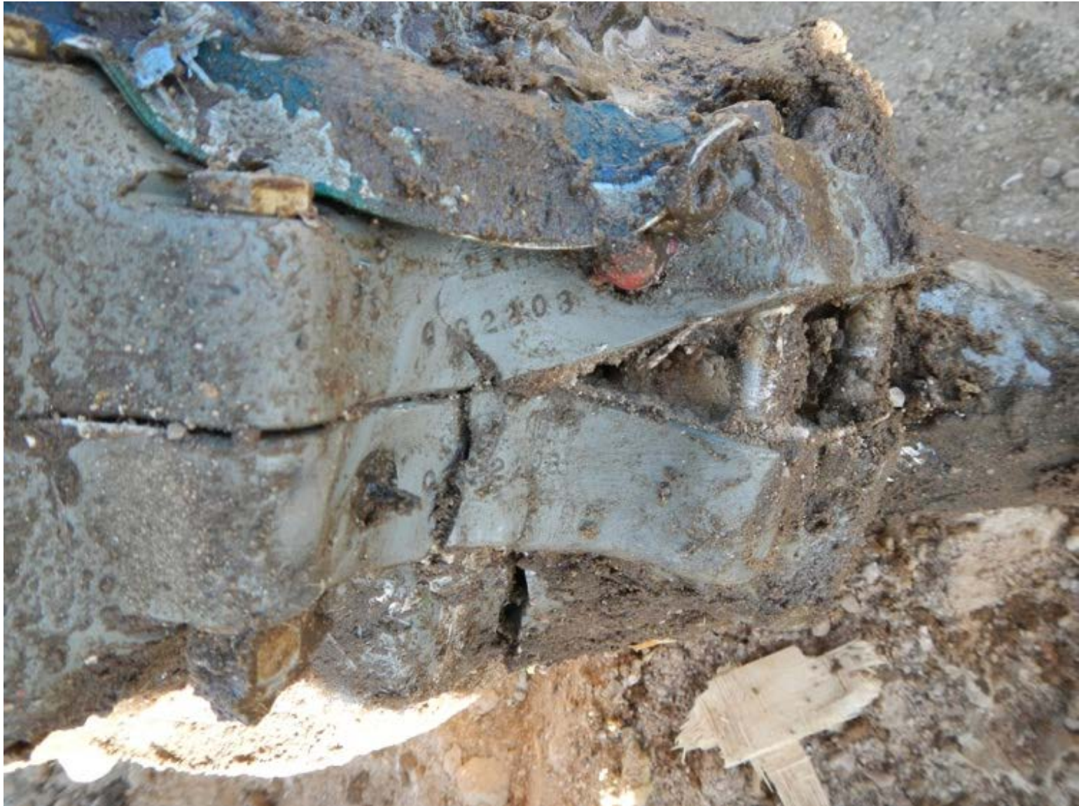
ASI-15-AF-81 Three bladed propeller hub; serial CG 2203
