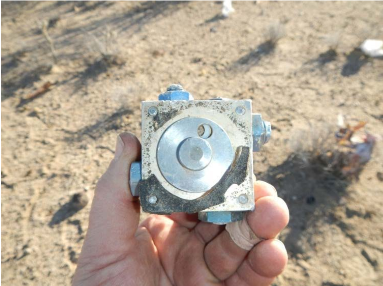
ASI-15-AF-55 Fuel selector valve port and rotor
