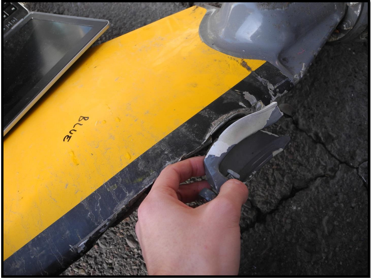
Figure 8-Blue Blade and Impact Damage
