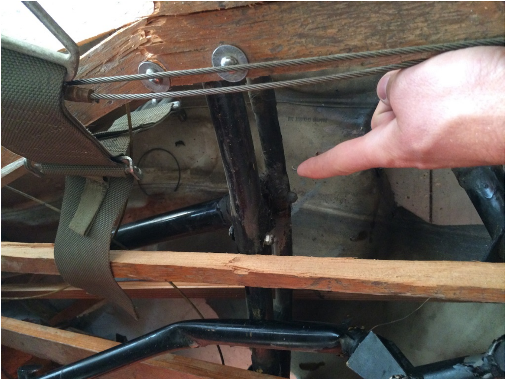
Photo 4 – Aft Fractured End of Control Tube
