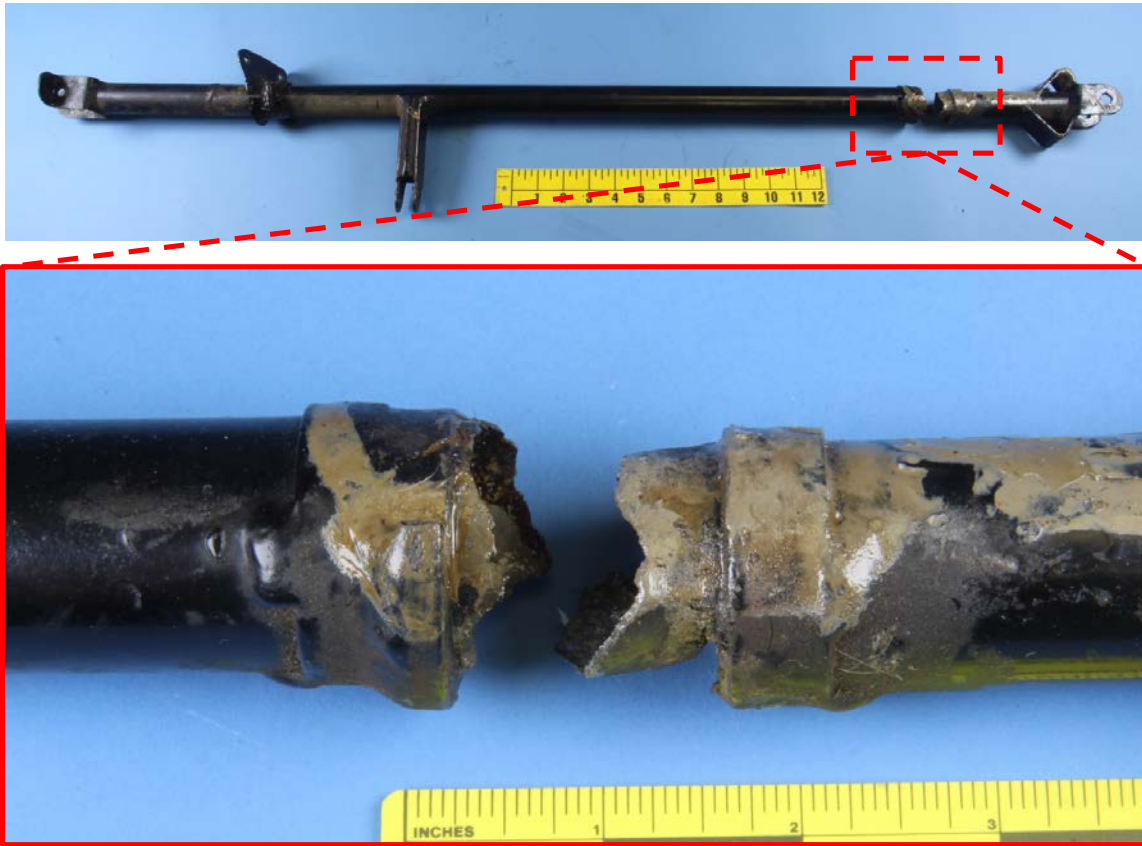
Figure 1: An overall photo of the separated control tube is shown in the top photo. The bottom photo shows a close-up photo of the separation in the control tube.
