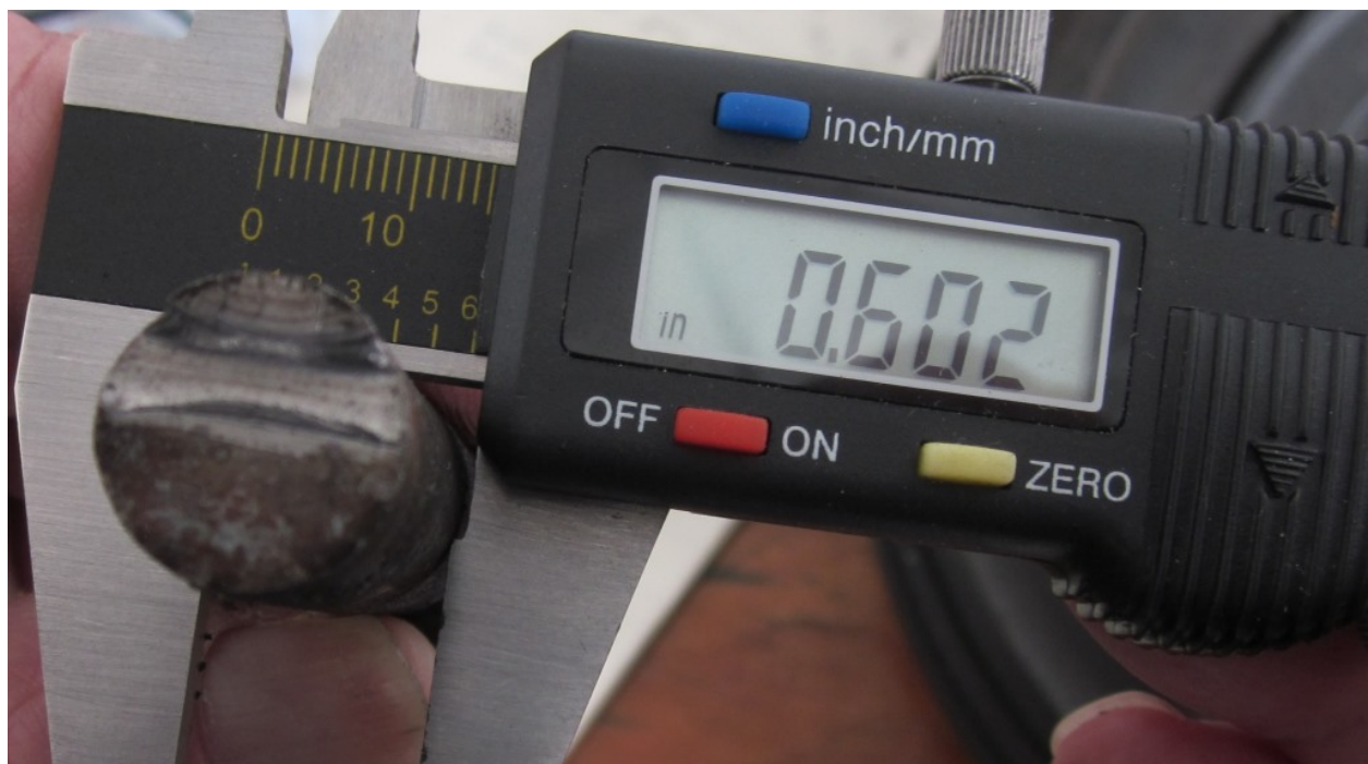
Figure 8 - Shaft Diameter Measurement (Note incorrect location of shaft in micrometer)
