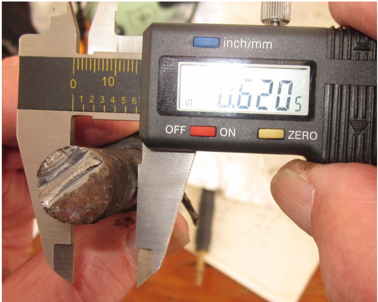
Figure 9 - Shaft Diameter Measurement (Note incorrect location of shaft in micrometer)
