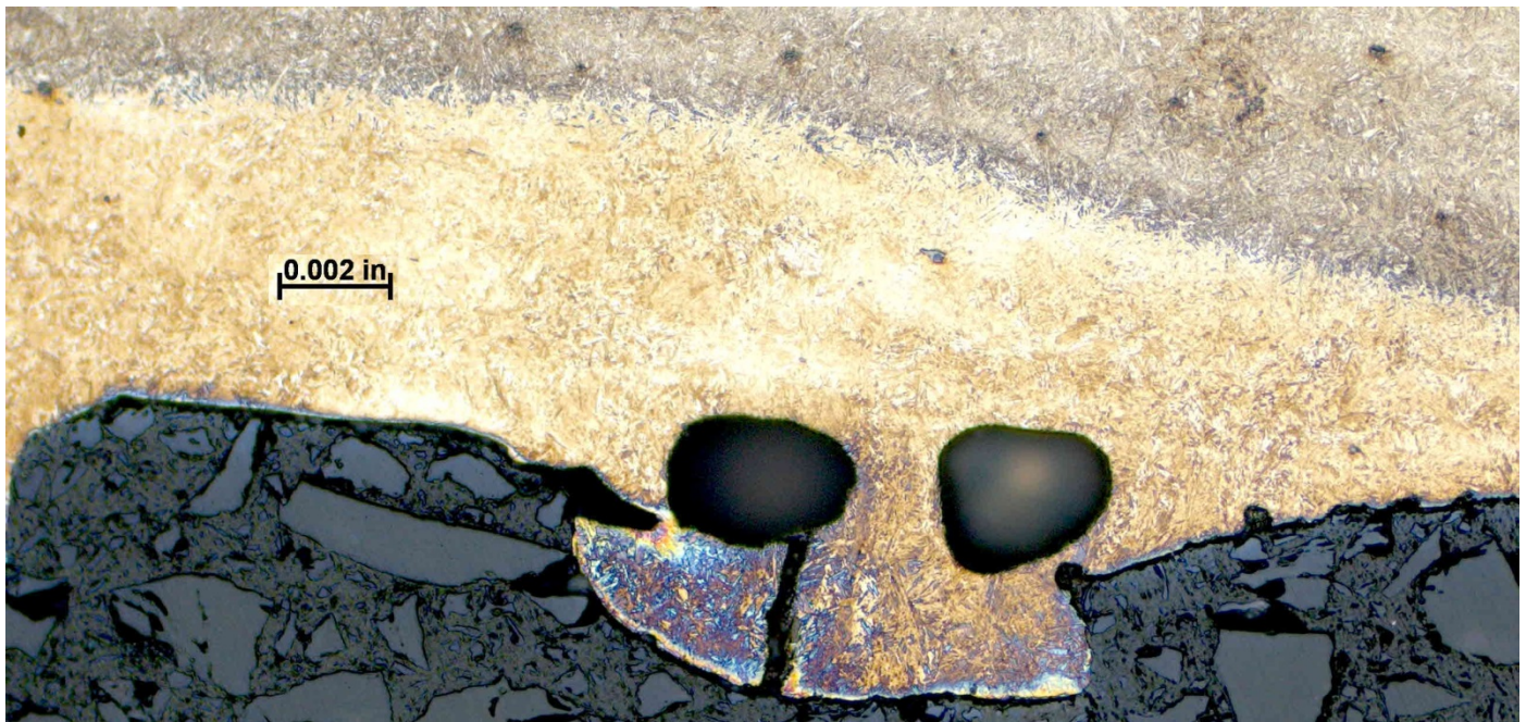
Figure 4. Nital etched metallographic section showing the white zone corresponding to the resolidified region and the fracture initiation area.
