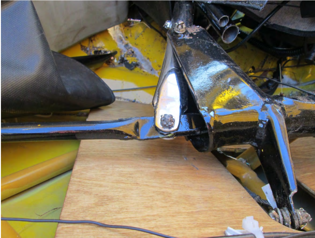
Photo 6 Front Elevator Control Connection
