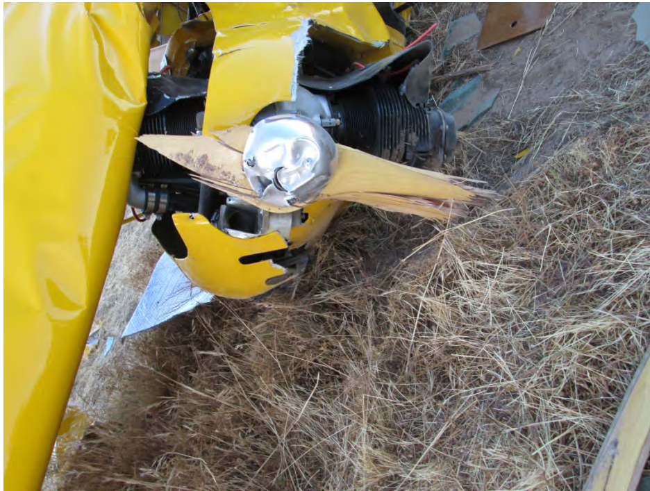
Photo 5 Shattered Propeller and Hub
