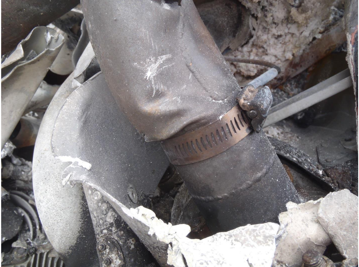
Photo 8. Right engine exhaust manifold.
