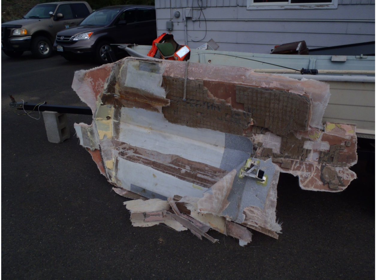
Photo 5. Interior view of the hull bottom wreckage.
