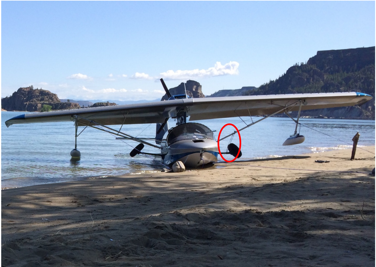
Photo 1. The airplane parked on the beach prior to takeoff, showing the left landing gear tied to the left wing lift-strut. (Courtesy Michael Robbins)
