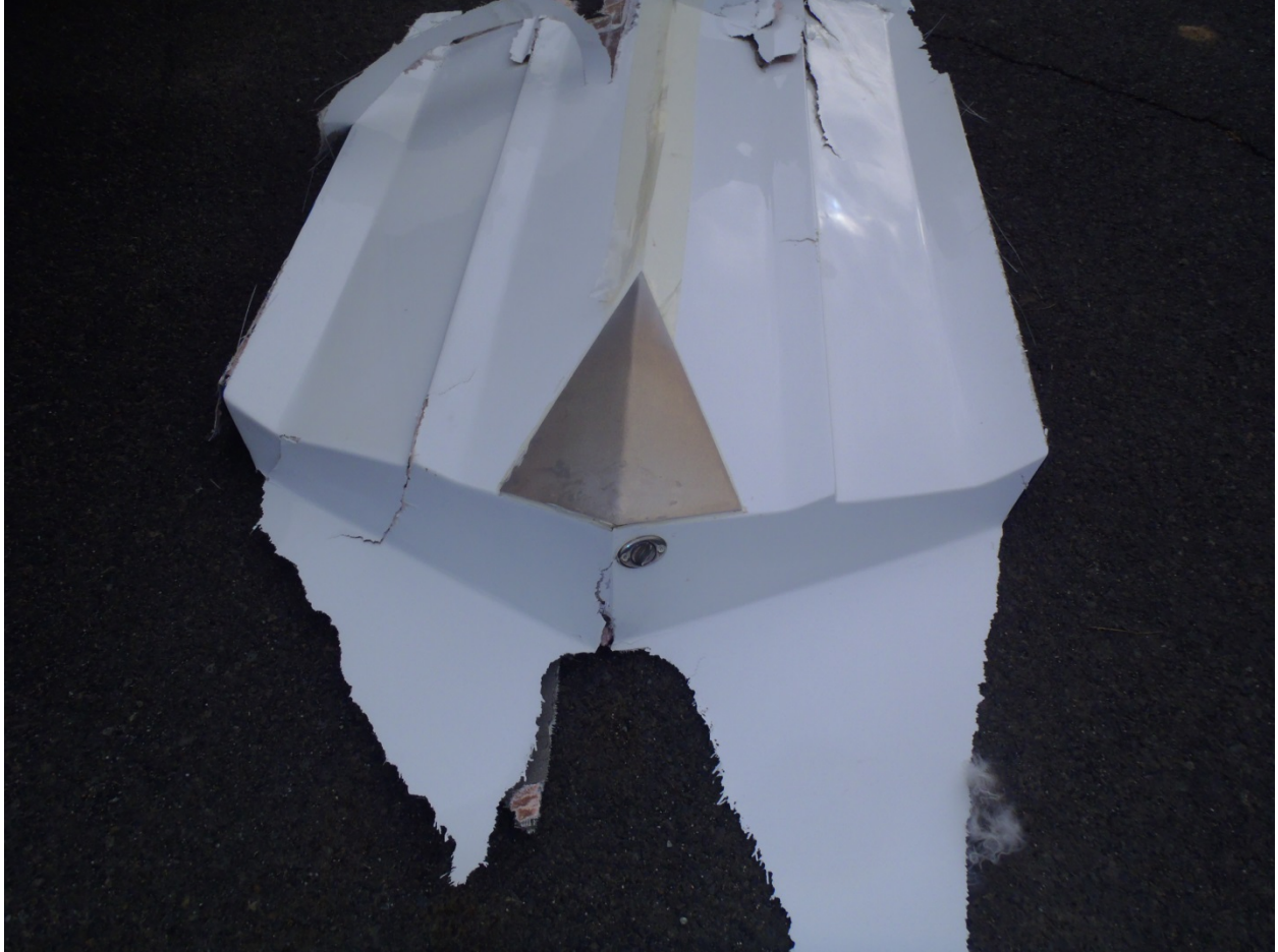
Photo 4. Exterior view of the airplane's hull bottom wreckage, viewed from the aft step forward.
