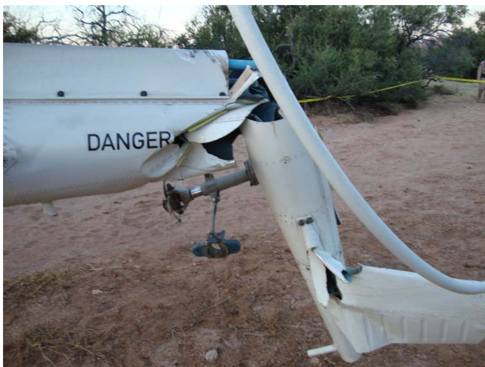
Figure 3. Marks on T/R Drive Shaft Cover from Gearbox deflection upward
