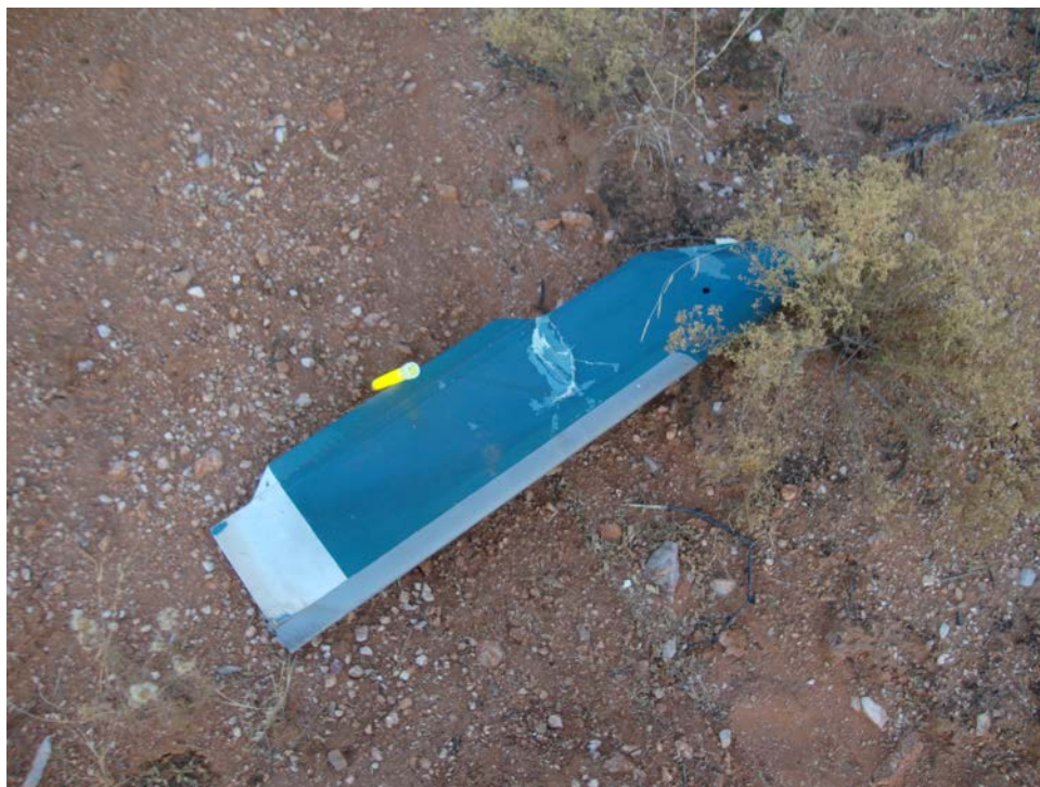
Figure 5. Damage to Tail Rotor (2)
