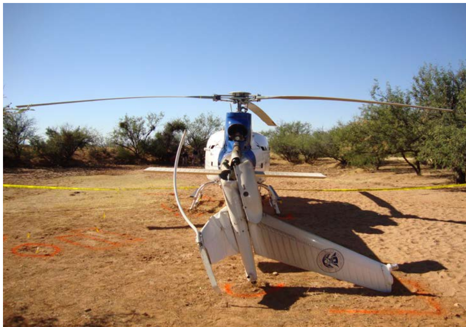
Figure 1. Damage to Tail Section (1)
