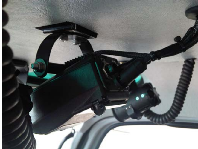
Figure 7. Appareo Vision 1000 Camera
