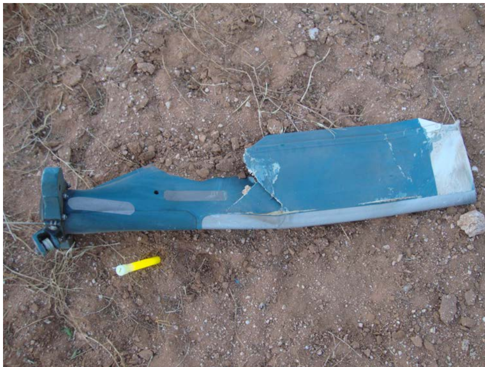
Figure 4. Damage to Tail Rotor (1)
