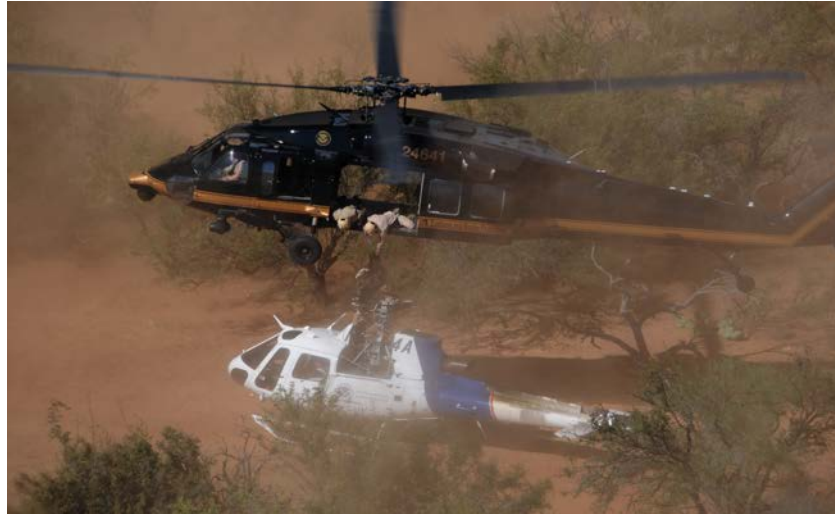
Figure 6. Aircraft Relocation for transport
