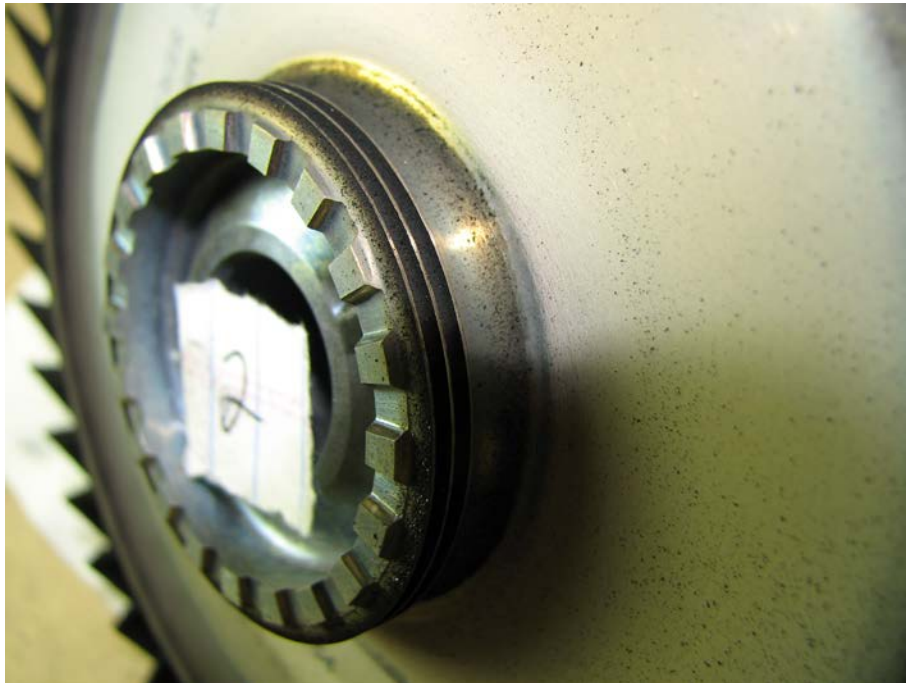
Figure 10 – 2nd Stage Turbine Wheel Curvic Coupling
