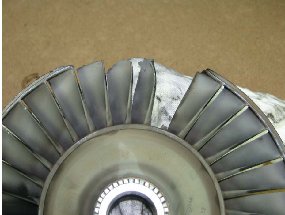
Figure 21 – 4th Stage Turbine Wheel
