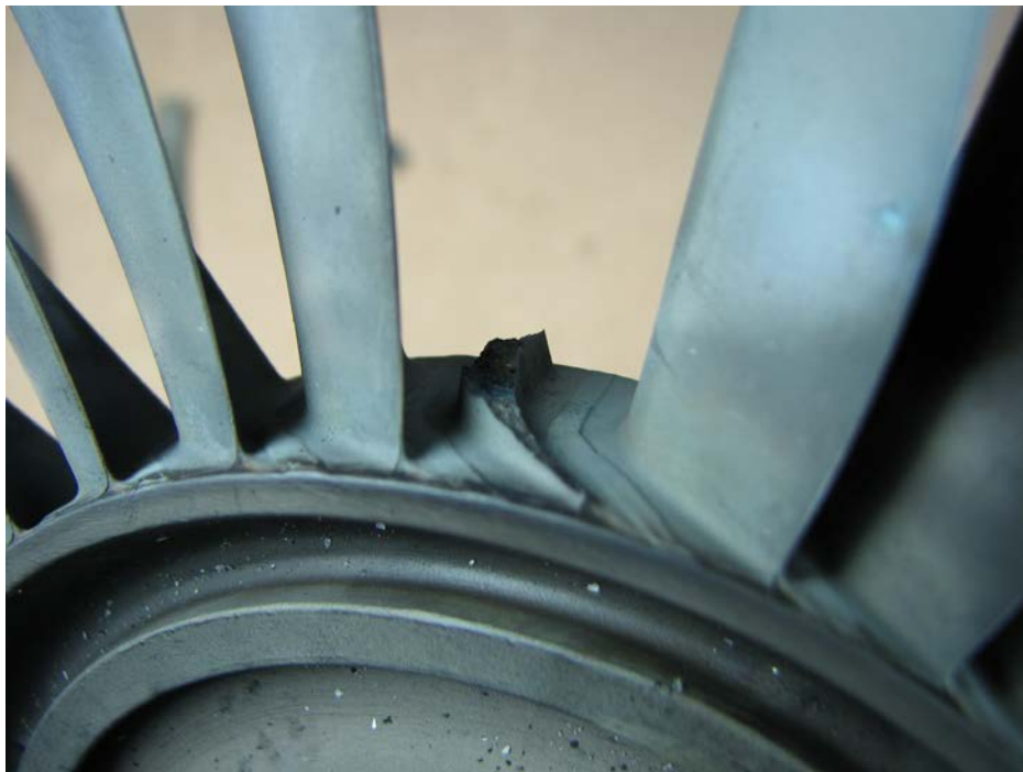
Figure 22 – 4 th Stage Turbine Wheel - Fractured Near the Inner Platform
