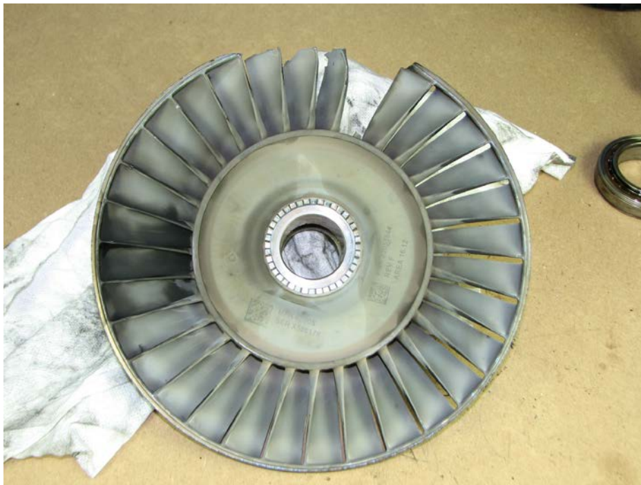
Figure 20 – 4th Stage Turbine Wheel
