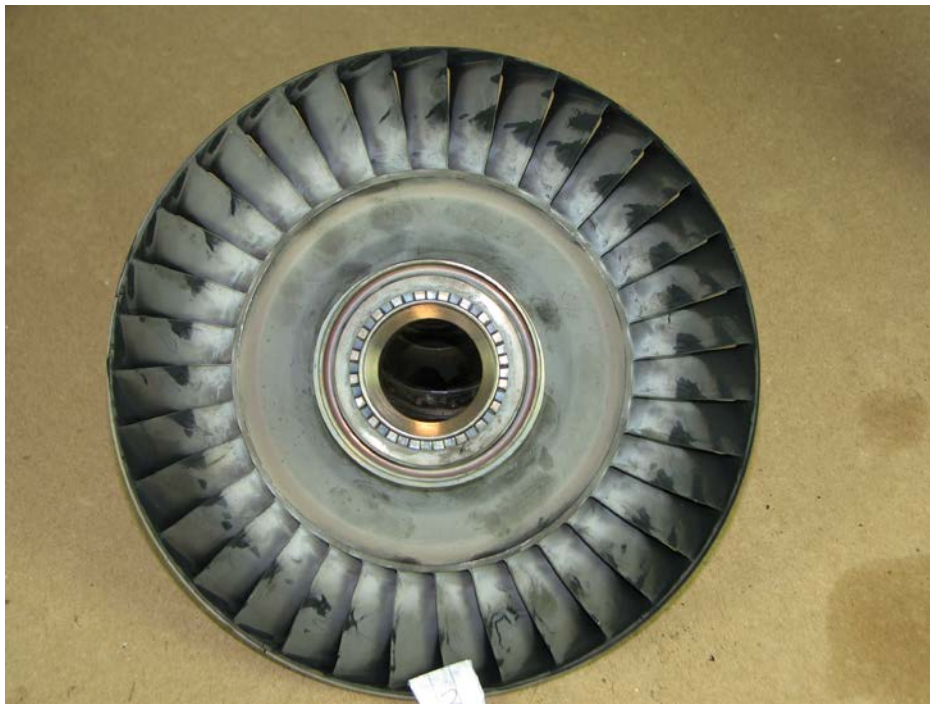
Figure 18 – 3 rd Stage Turbine Wheel
