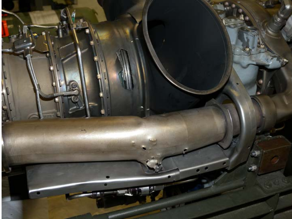
Figure 11 – Uncontained Particle Damage
