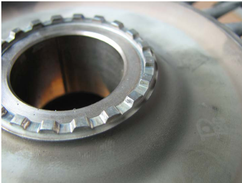
Figure 24 – 4th Stage Turbine Wheel – Curvic Teeth
