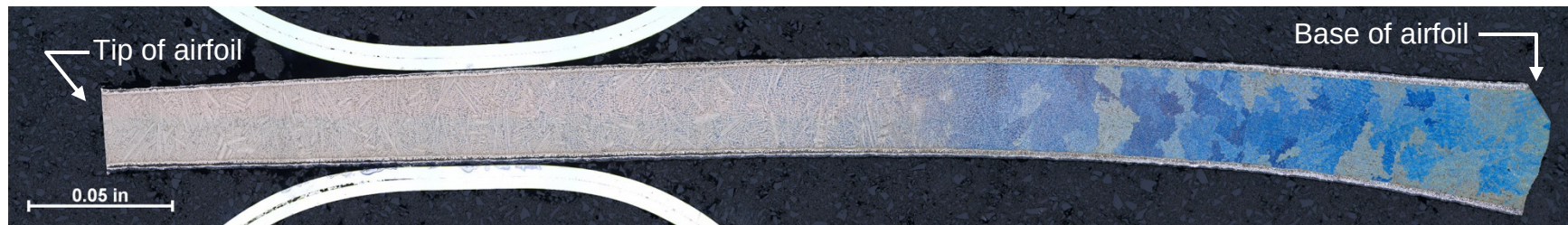
Figure 8: Metallographic cross section of a first-stage turbine wheel airfoil adjacent and parallel to the trailing edge from the base to the tip of the airfoil.
