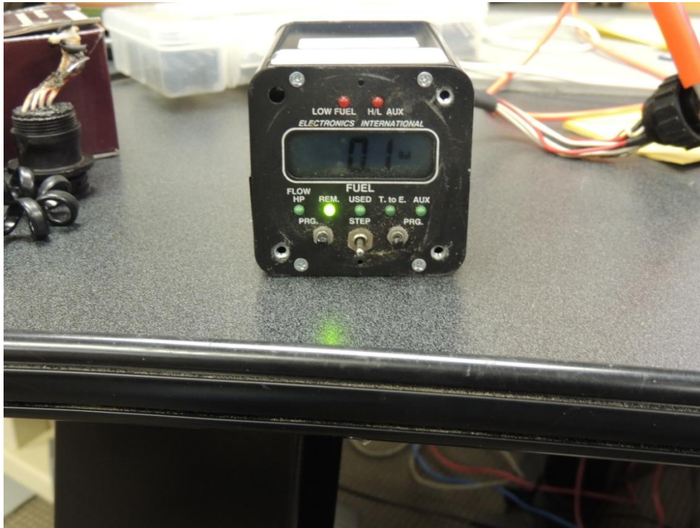
Figure 2. Fuel remaining tab of FP-5L with a value of 0.1 gallons.
