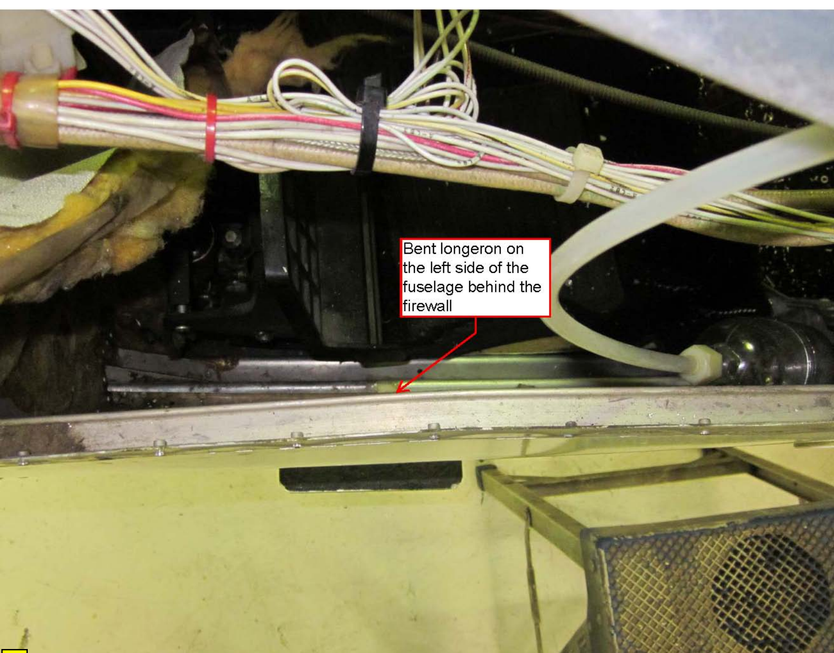
Photo 3. Bent Longeron Left Side (Provided by FAA)
