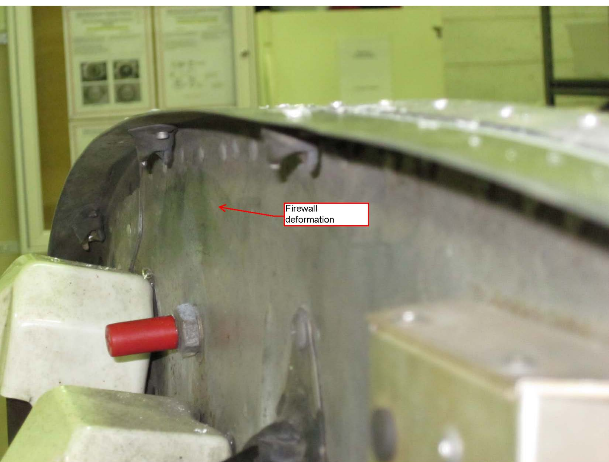
Photo 5. Firewall Deformation (Provided by FAA)
