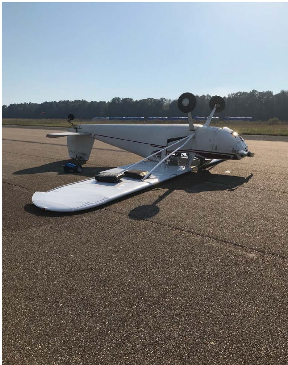
Photo 1 – View of damaged left wing lift strut and rudder (courtesy of the FAA)
