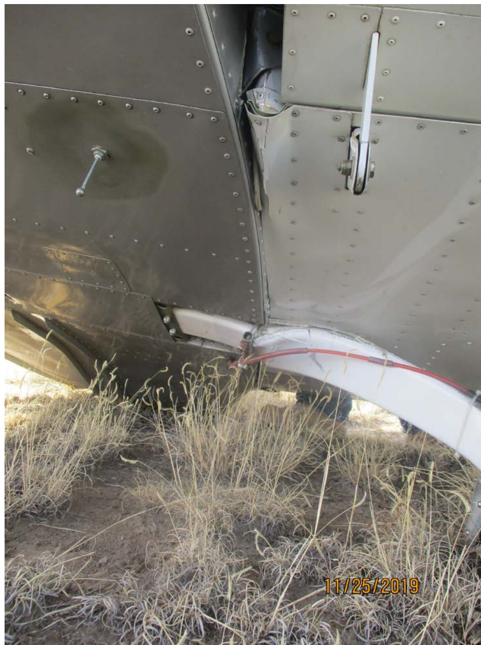
Photo 2 - View of damage to the inboard right wing (Courtesy of FAA)
