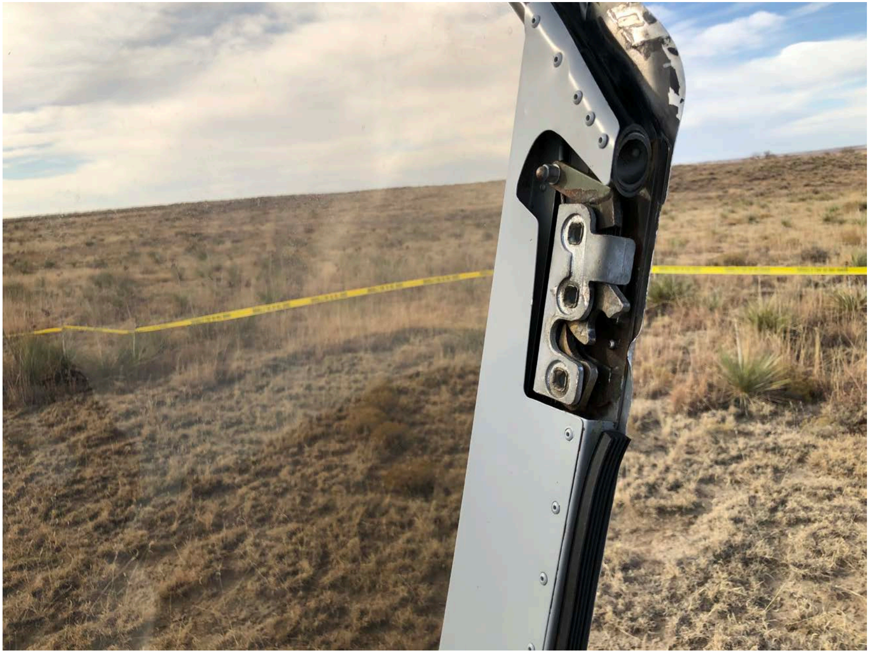
Photo 4 – View of the of the right side canopy handle and catch and lever (Courtesy of FAA)
