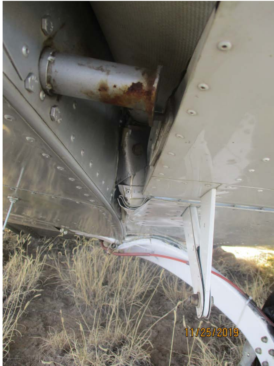
Photo 1 – View of damage to the inboard right wing (Courtesy of FAA)
