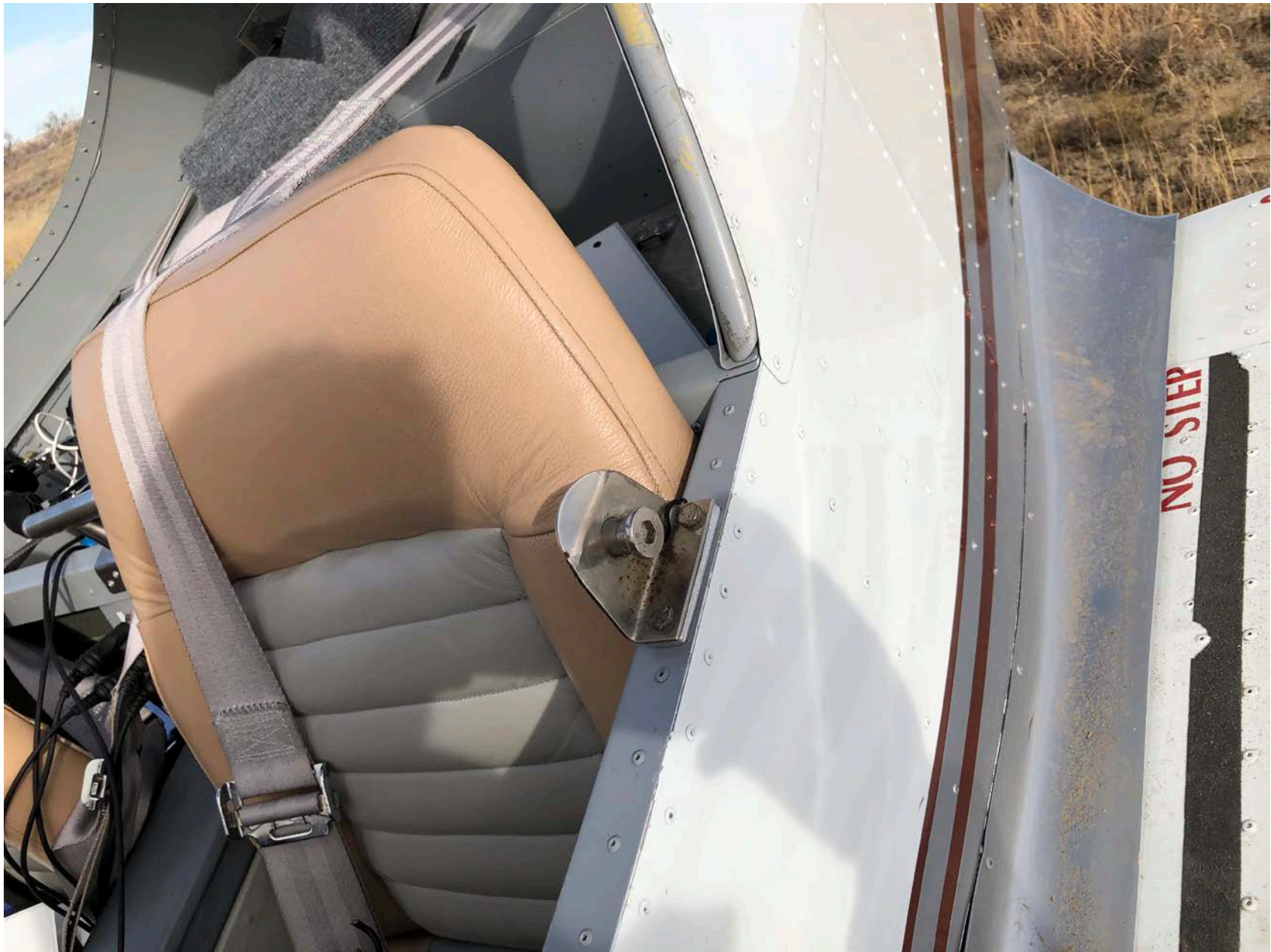
Photo 3 – View of the left side canopy latch (Courtesy of FAA)
