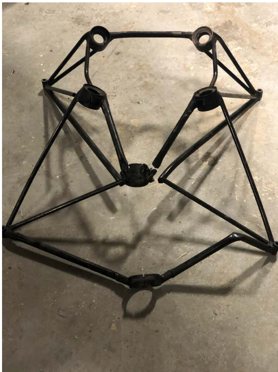
Photo 2 – View of damage to engine mount (Courtesy of Operator)
