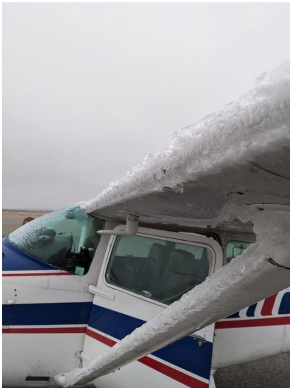
Photo 2 - View of airplane with ice (photo courtesy of the FAA)
