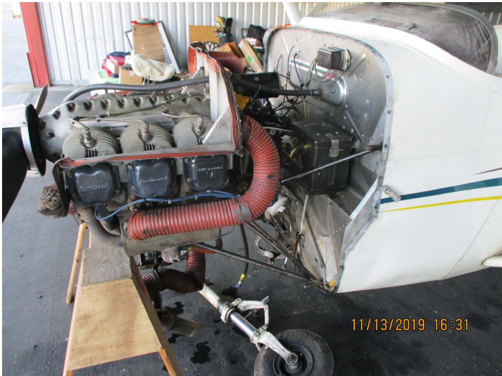
Photo 1 – View of damage to the lower left engine mount (Courtesy of FAA)
