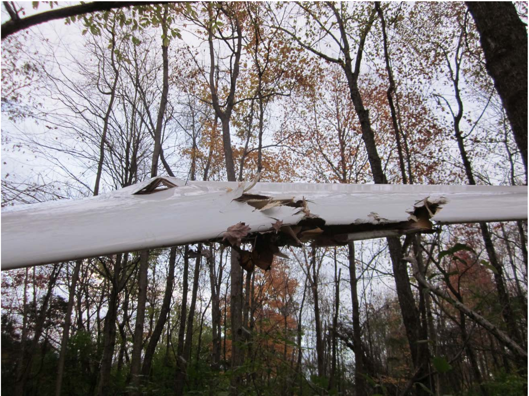
Photo 2 – Close-up view of damaged left wing (courtesy of FAA)
