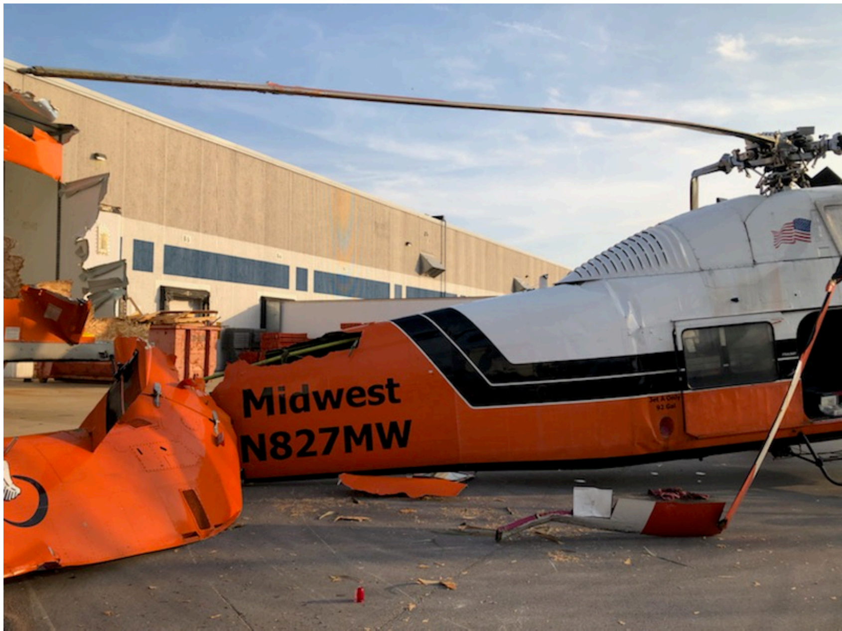
Photo 1 – View of damaged tailboom and trailer (courtesy of the FAA)
