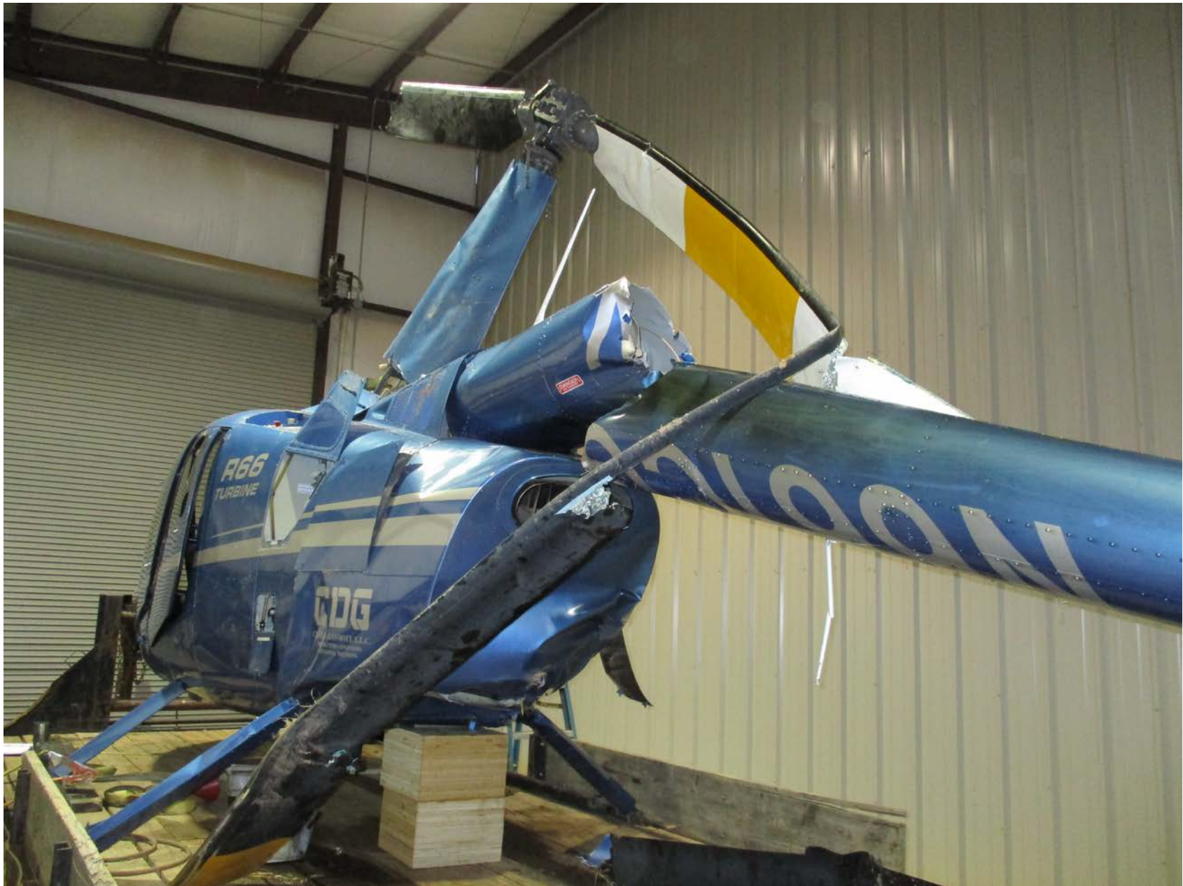
Photo 1 – View of damage to the tail rotor driveshaft, fuselage and main rotor blades (Courtesy of FAA)
