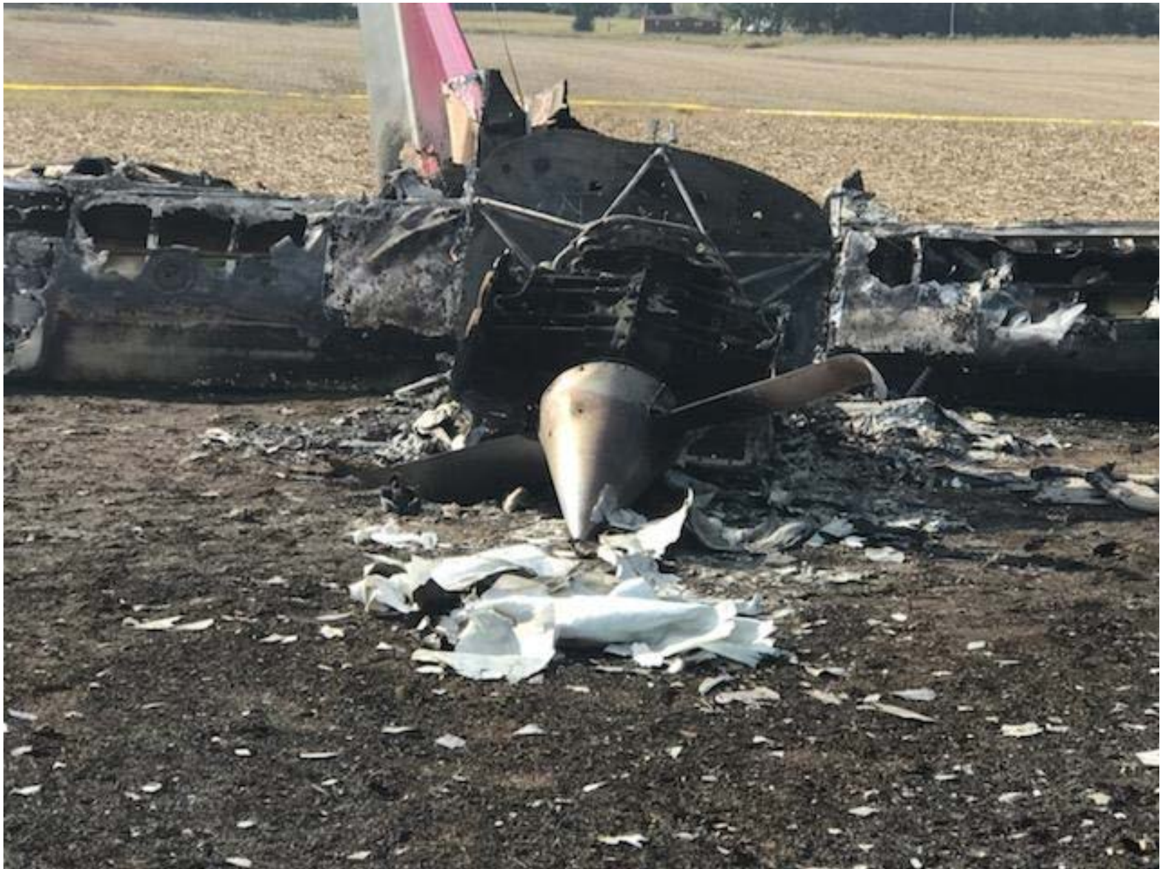
Photo 1 – View of fire damage to the airplane (Courtesy of FAA)
