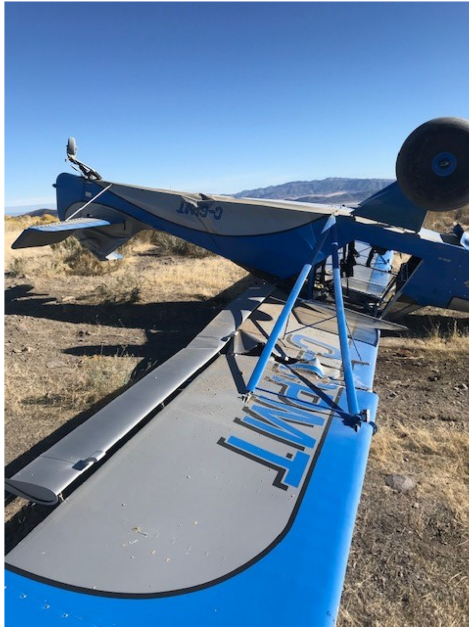
Photo 1 – View of damaged left wing, tailcone, and rudder (courtesy of the FAA)
