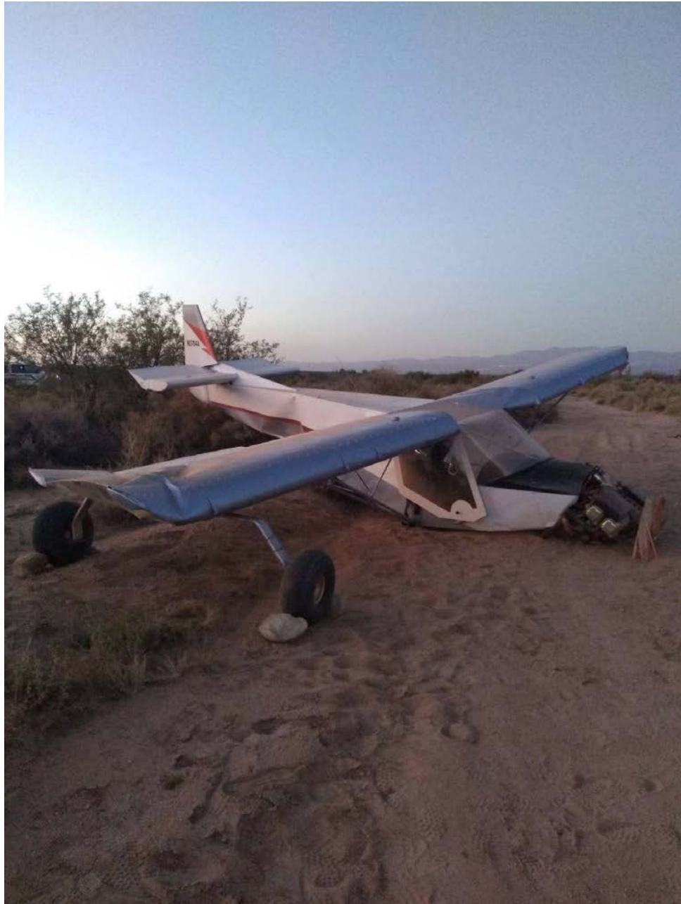
Photo 2 – View of damaged fuselage and right wing (Photo courtesy of the FAA)
