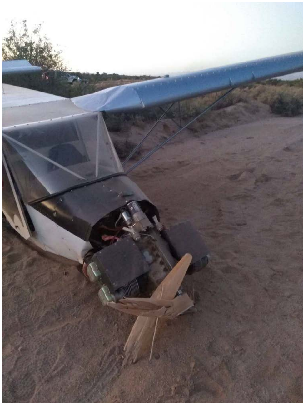
Photo 1 – View of damaged wooden propeller (Photo courtesy of the FAA)
