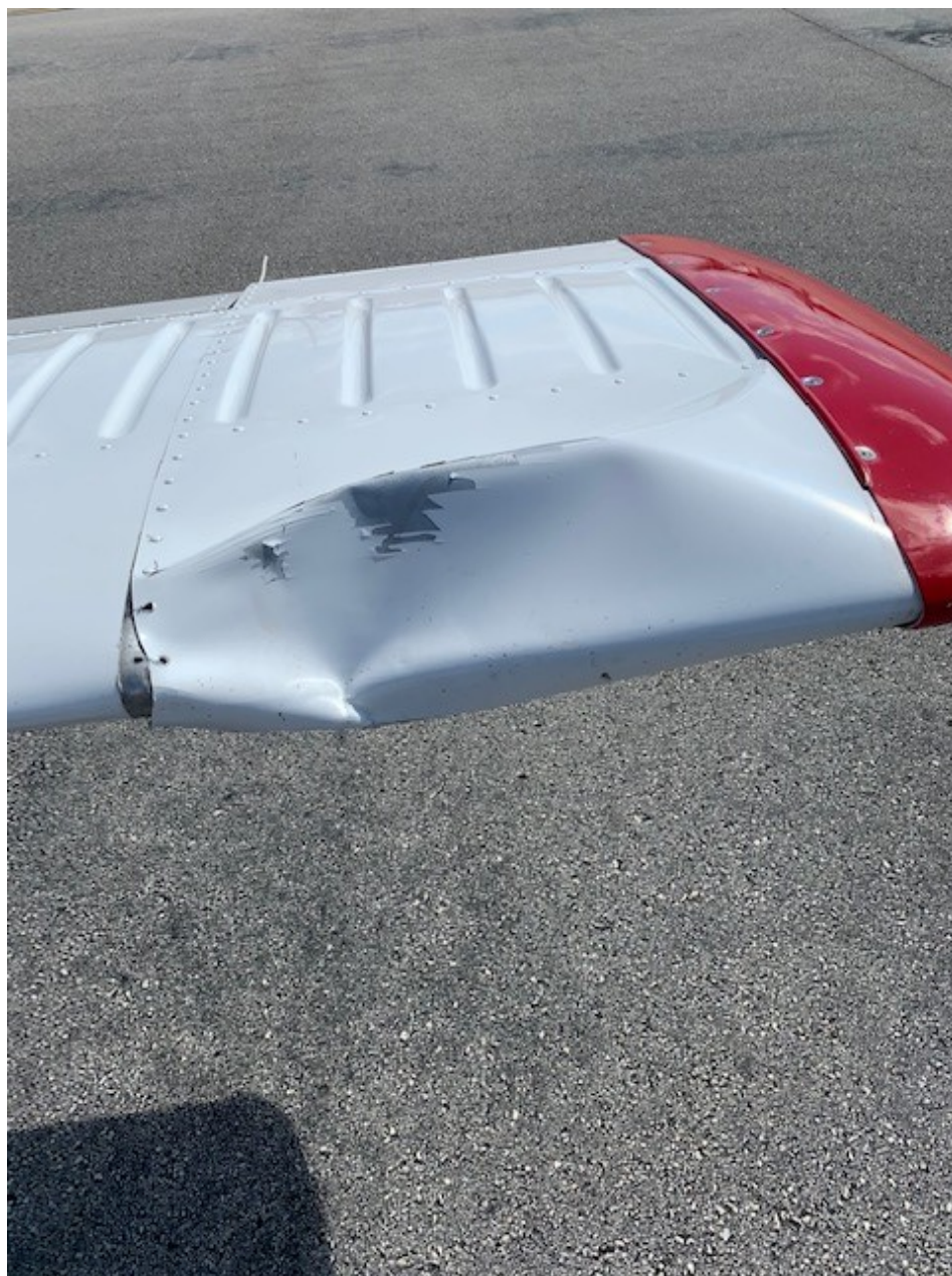
Photo 1 – View of stabilator damage (photo courtesy of the flight instructor)
