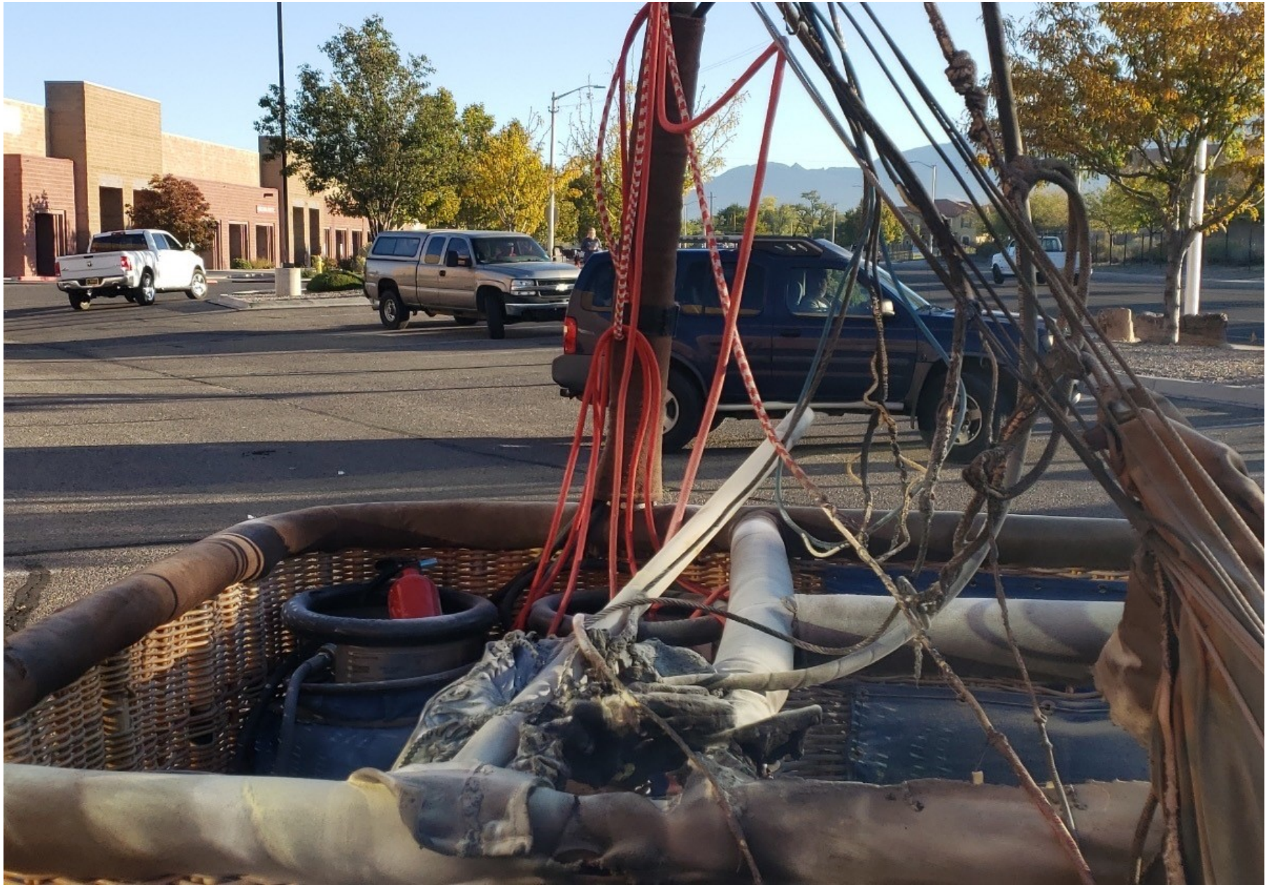
Photo 3 – View of damage to the basket's cables (Courtesy of FAA)
