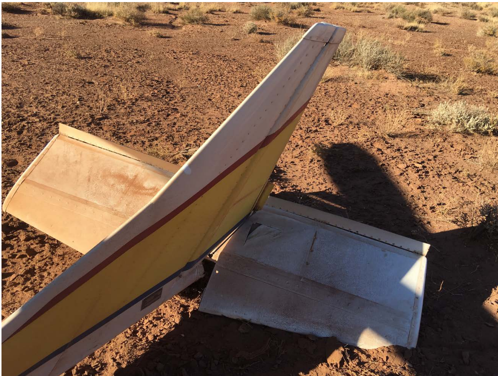
Photo 1 – View of damaged horizontal stabilizer (courtesy of the pilot)
