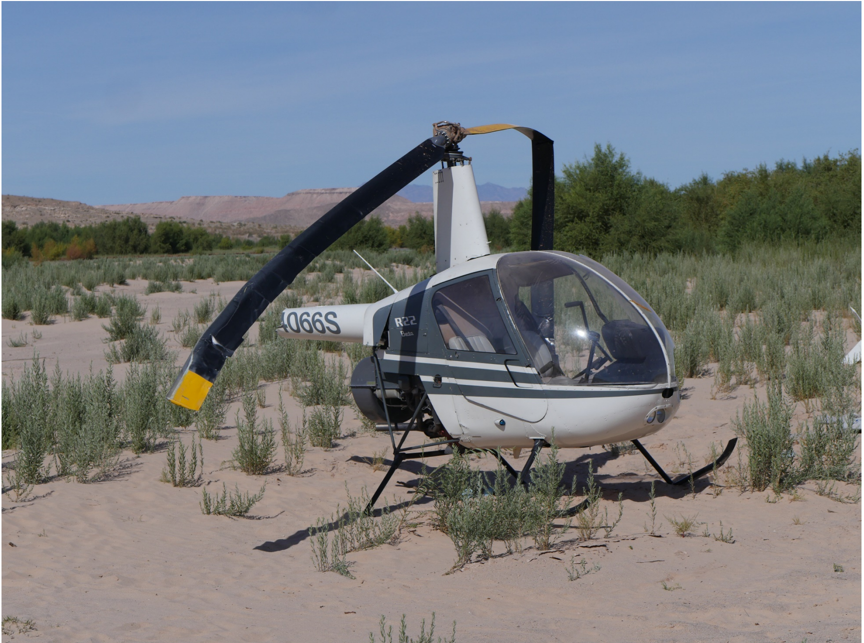
Photo 1 – View of damaged tailboom (Photo courtesy of the FAA)
