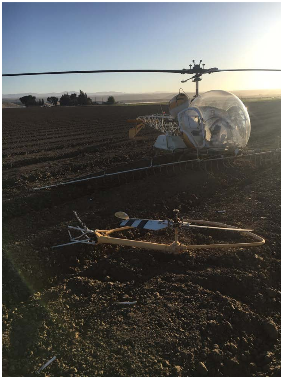
Photo 1 – View of tailboom damage (photo courtesy of unknown)
