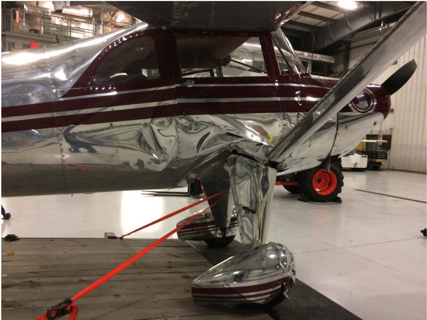
Photo – View of damaged lower fuselage (courtesy of the FAA)
