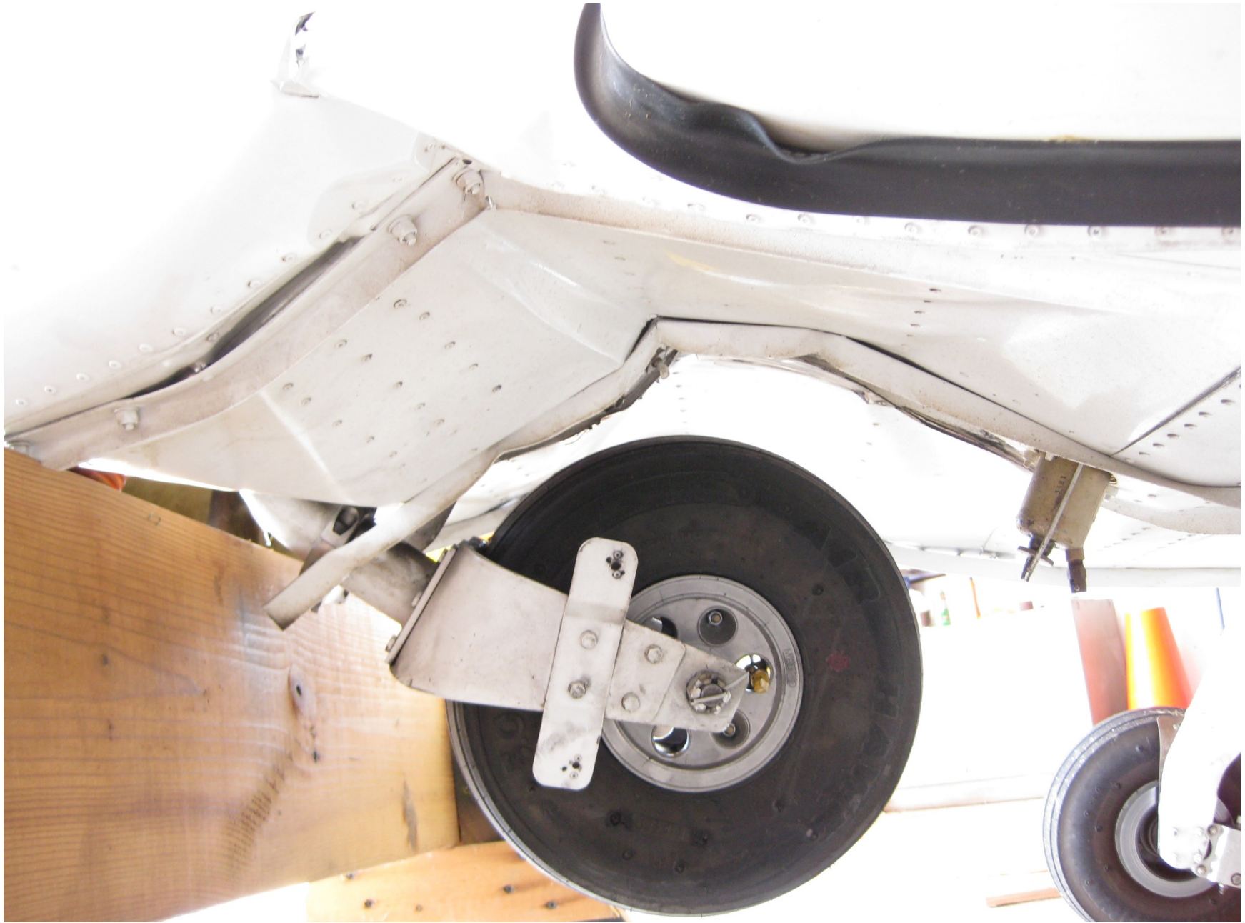
Photo 1 – View of collapsed nose landing gear and damaged fuselage (Photo courtesy of the FAA)
