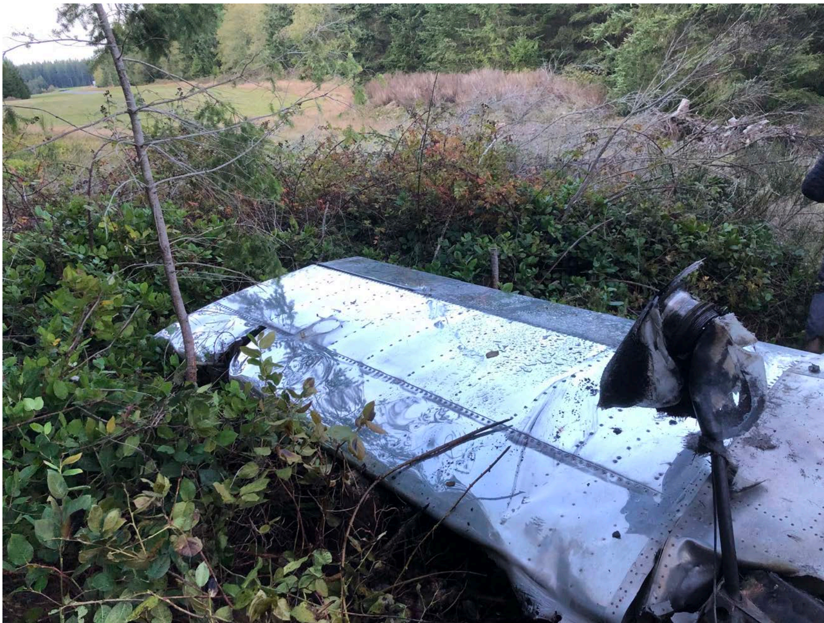
Photo 1 – View of left wing damage (photo courtesy of local law enforcement)
