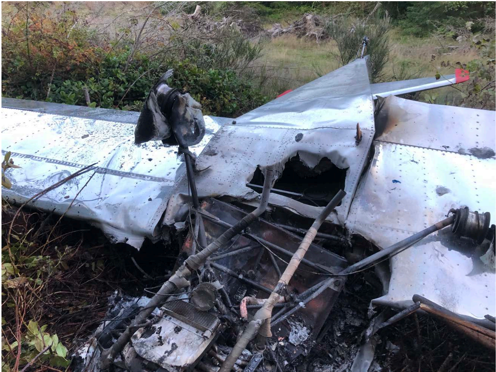
Photo 2 - View of post fire fuselage damage (photo courtesy of local law enforcement)
