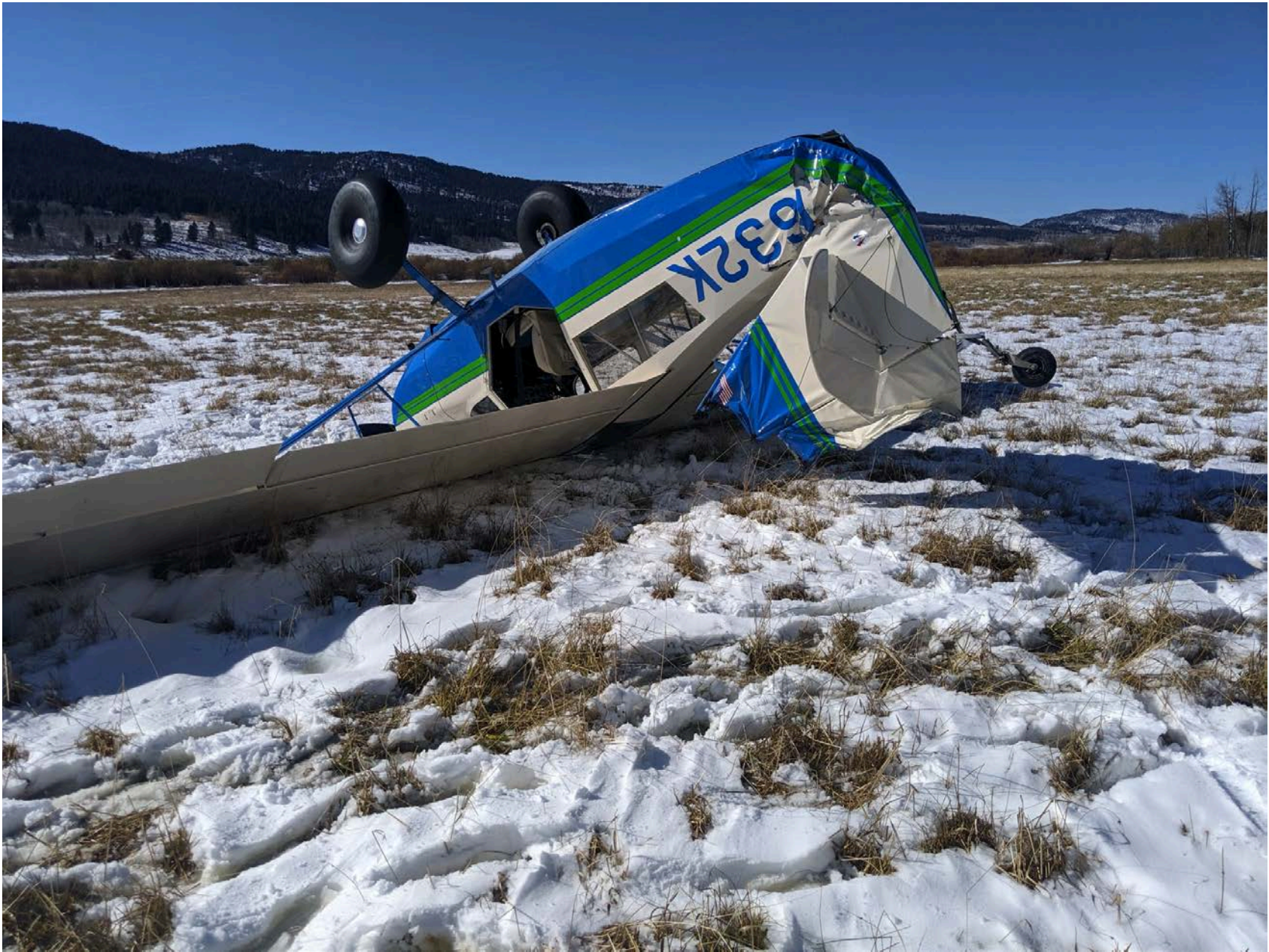
Photo 1 – View of fuselage and empennage damage (photo courtesy of unknown)
