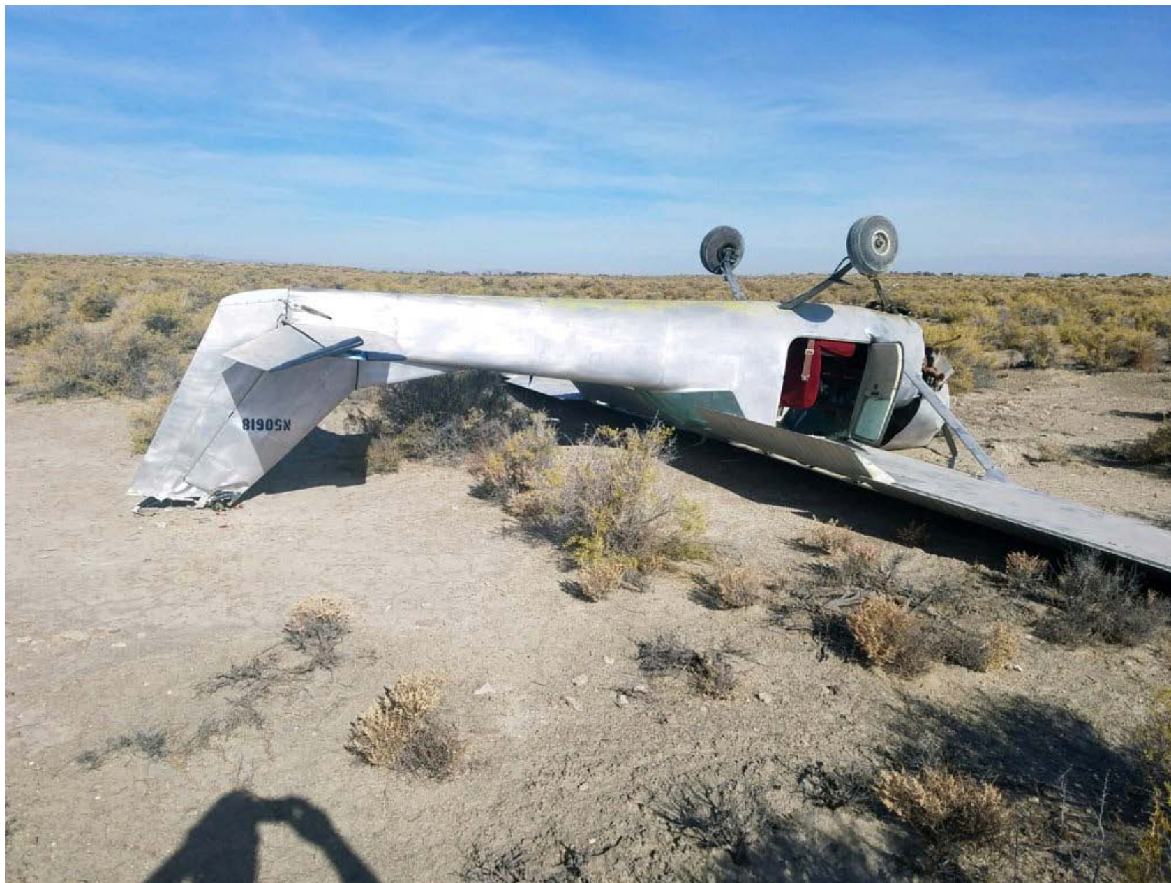
Photo 1 – View of damage to the airplane’s vertical stabilizer and rudder (Courtesy of FAA)
