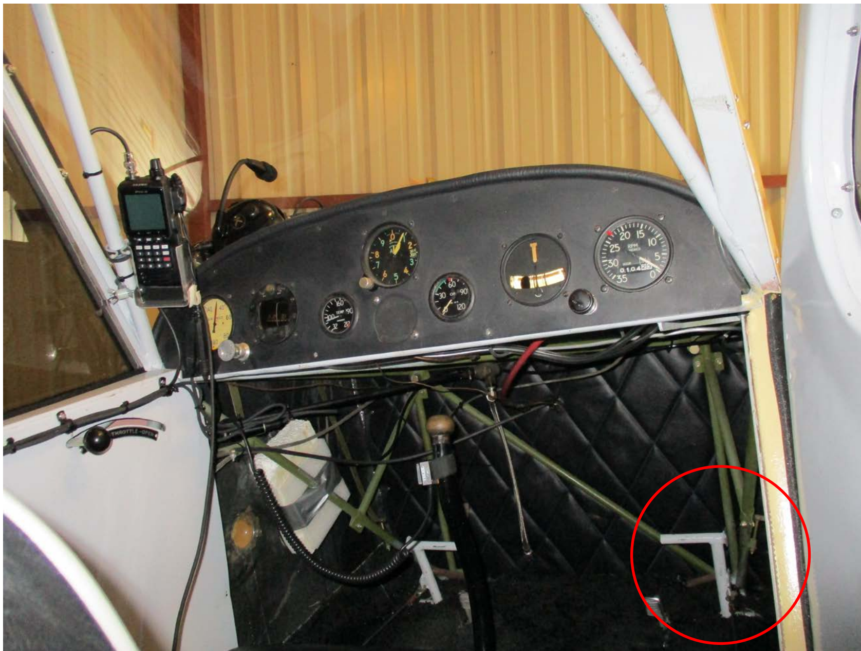
Photo 3 – View of right rudder pedal in the front seat of the cockpit (courtesy of the FAA)
