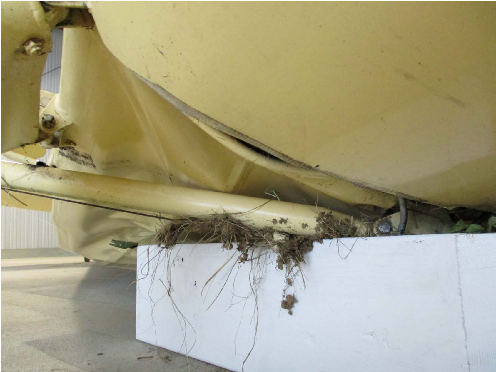
Photo 1 – Bottom view of airplane's damaged lower, right fuselage (courtesy of the FAA)
