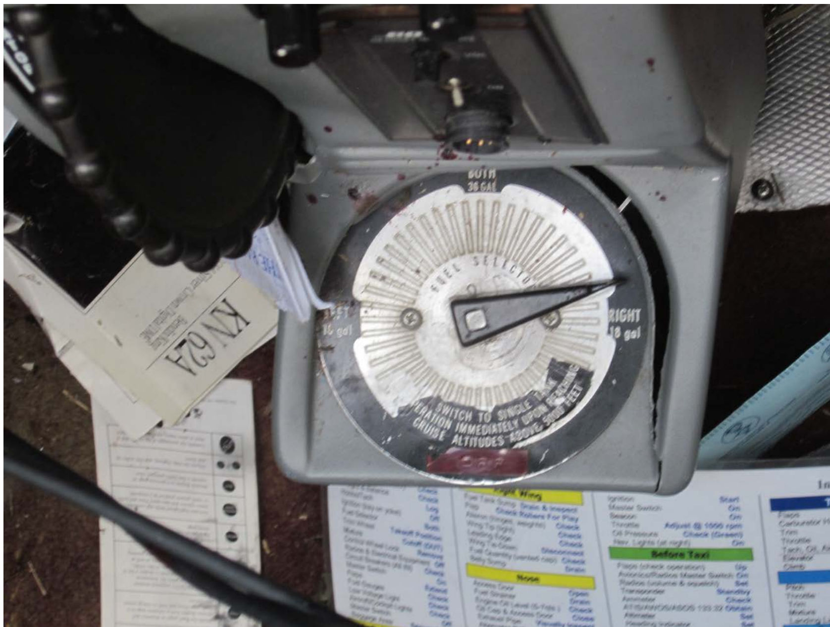
Photo 3 - View of selector valve lever on right fuel tank (photo courtesy of the FAA)
