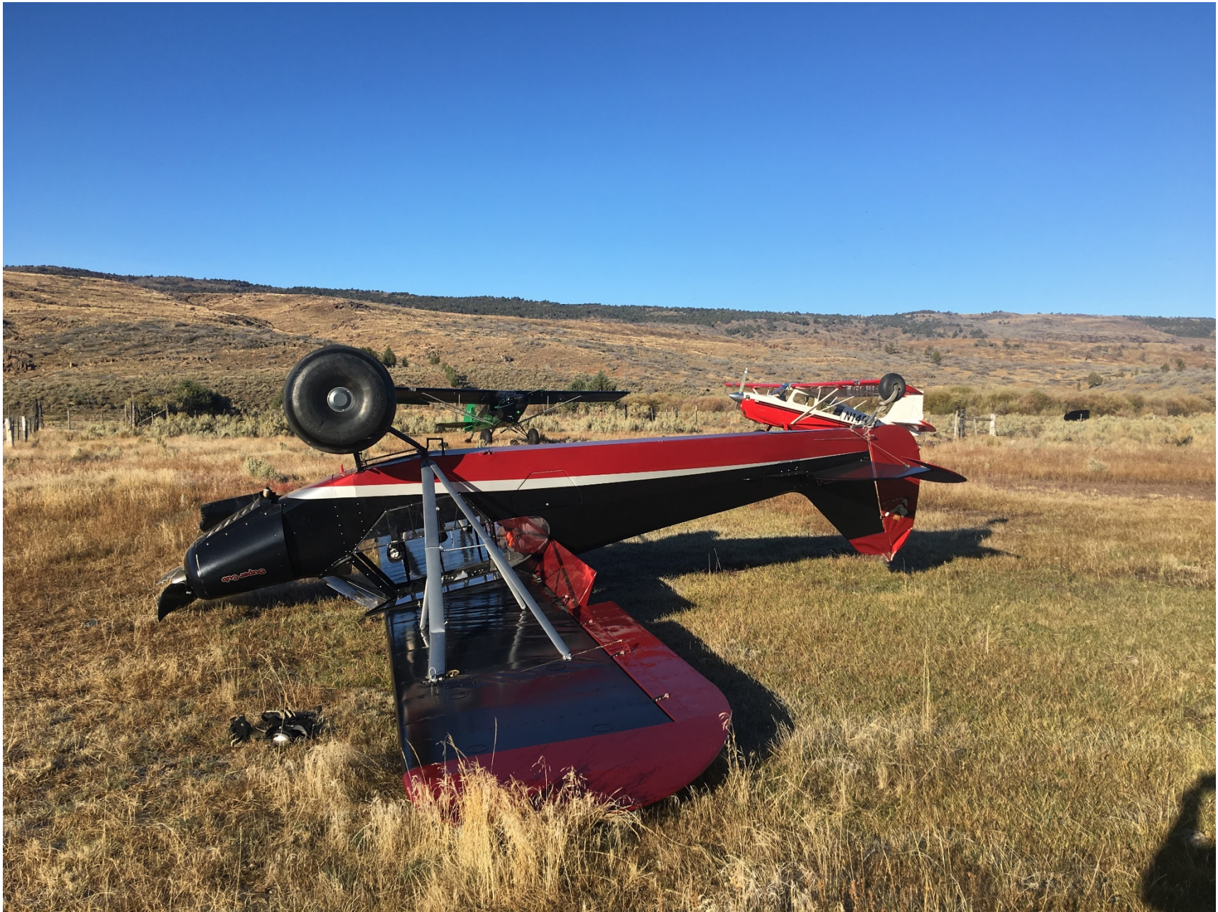
Photo 1 – View of damaged right wing lift strut and rudder of inverted airplane (Photo courtesy of the pilot)
