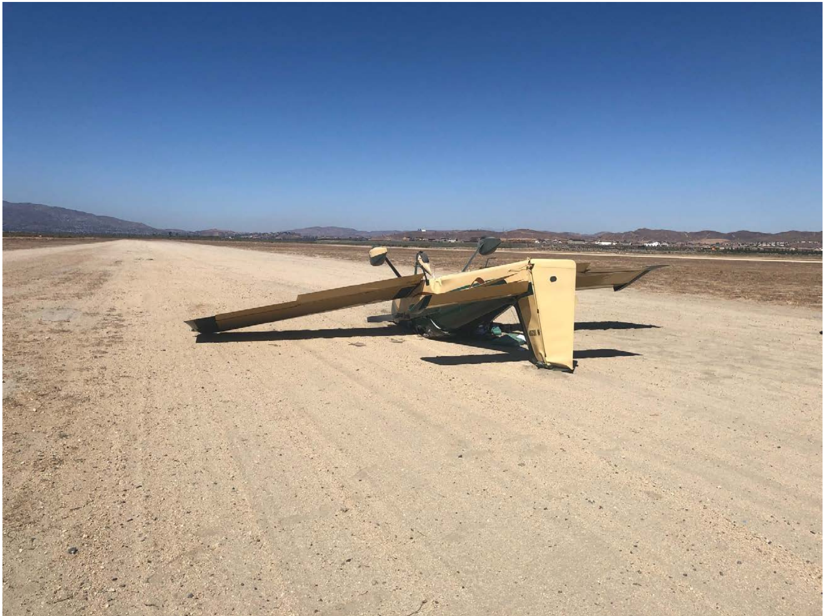
Photo 1 – View of rudder and fuselage damage (photo courtesy of the FAA)
